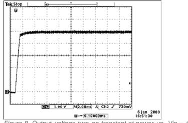
Figure 8. Output-voltage turn-on transient at power-up. Vin = 48V, Iout = 5A.
