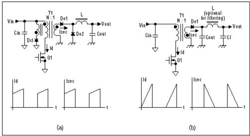
Figure 2. Forward (a) and flyback (b) power topologies.
