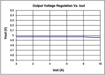
Figure 10. Output-voltage regulation.
