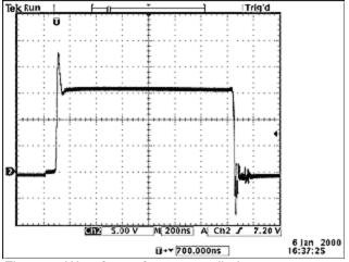
Figure 7. Waveform after output diode.
