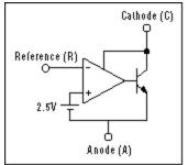
Figure 6. Simplified block diagram of the shunt regulator.
