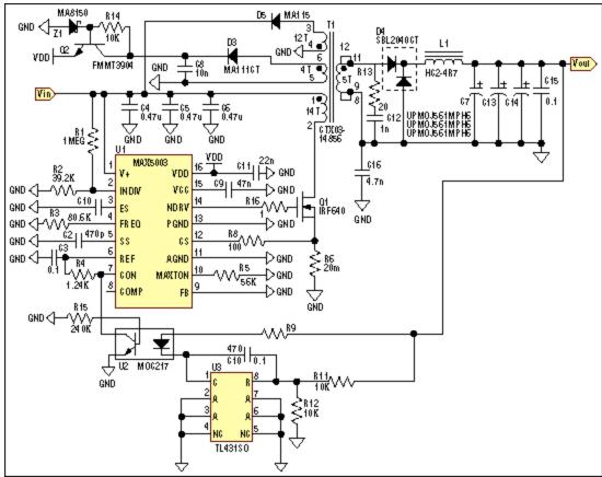
Figure 1. Schematic diagram of ≈48V in and 5V out @ 10A isolated power supply.
