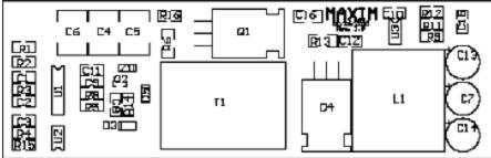
Figure 12. Component placement of the FWD0510 power supply; note that Q1 and D4 are placed on the bottom side, where their metal tabs are exposed to the heatsink plate.
