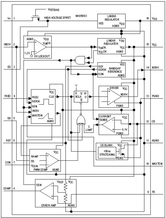
Figure 3. MAX5003 block diagram.
