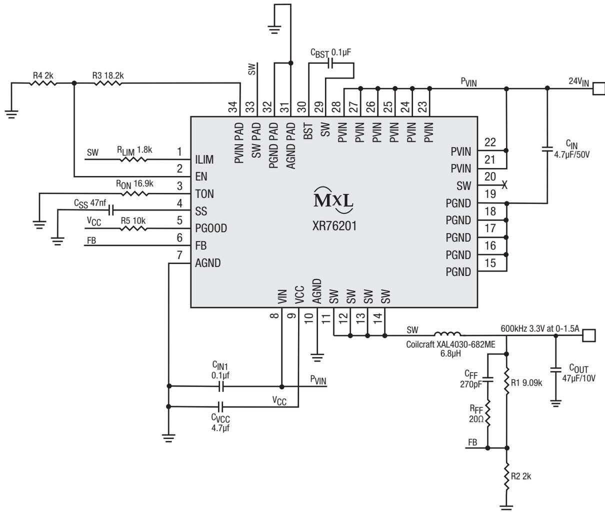
Figure 24. Application Circuit
