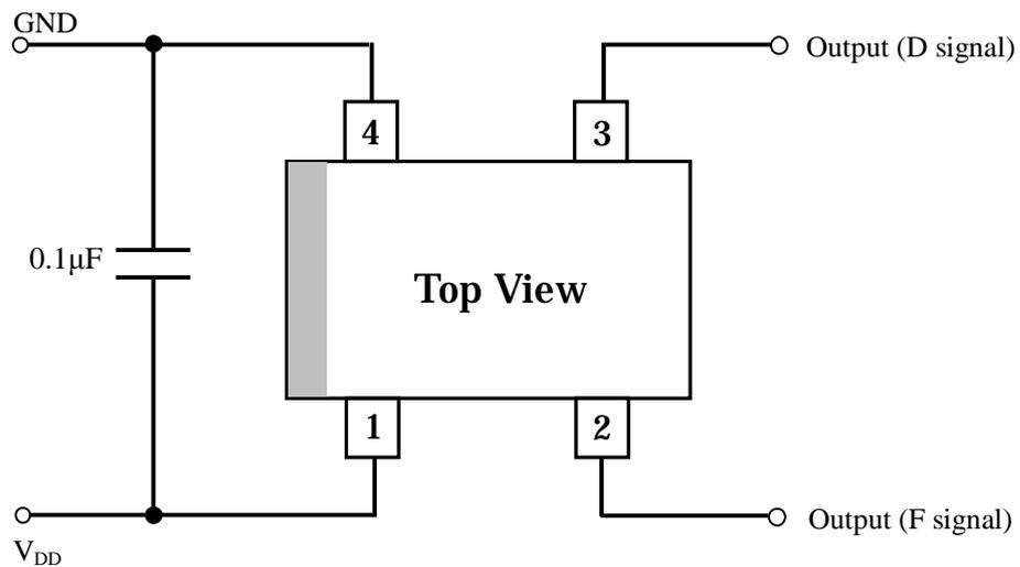
Figure 10. Recommended external circuit
