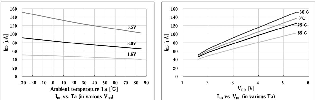
Figure 7. Temperature dependence of current consumption
