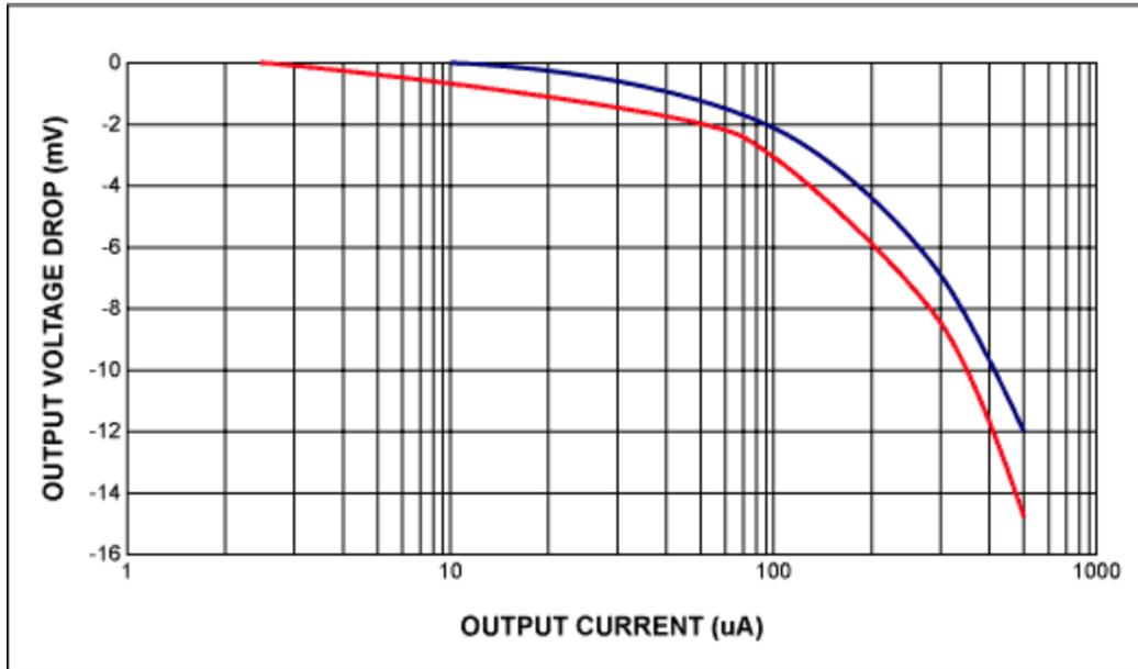
Figure 2. The load-regulation error of the circuit's output.
