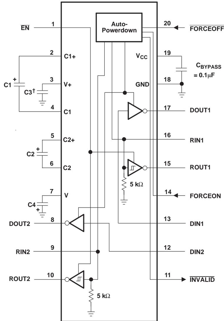
† C3 can be connected to V<sub>CC</sub> or GND.
