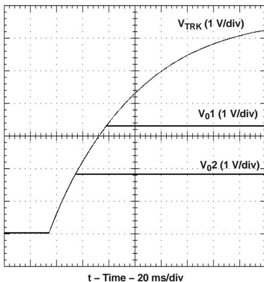
Figure 15. Simultaneous Power Up With Auto-Track Control
