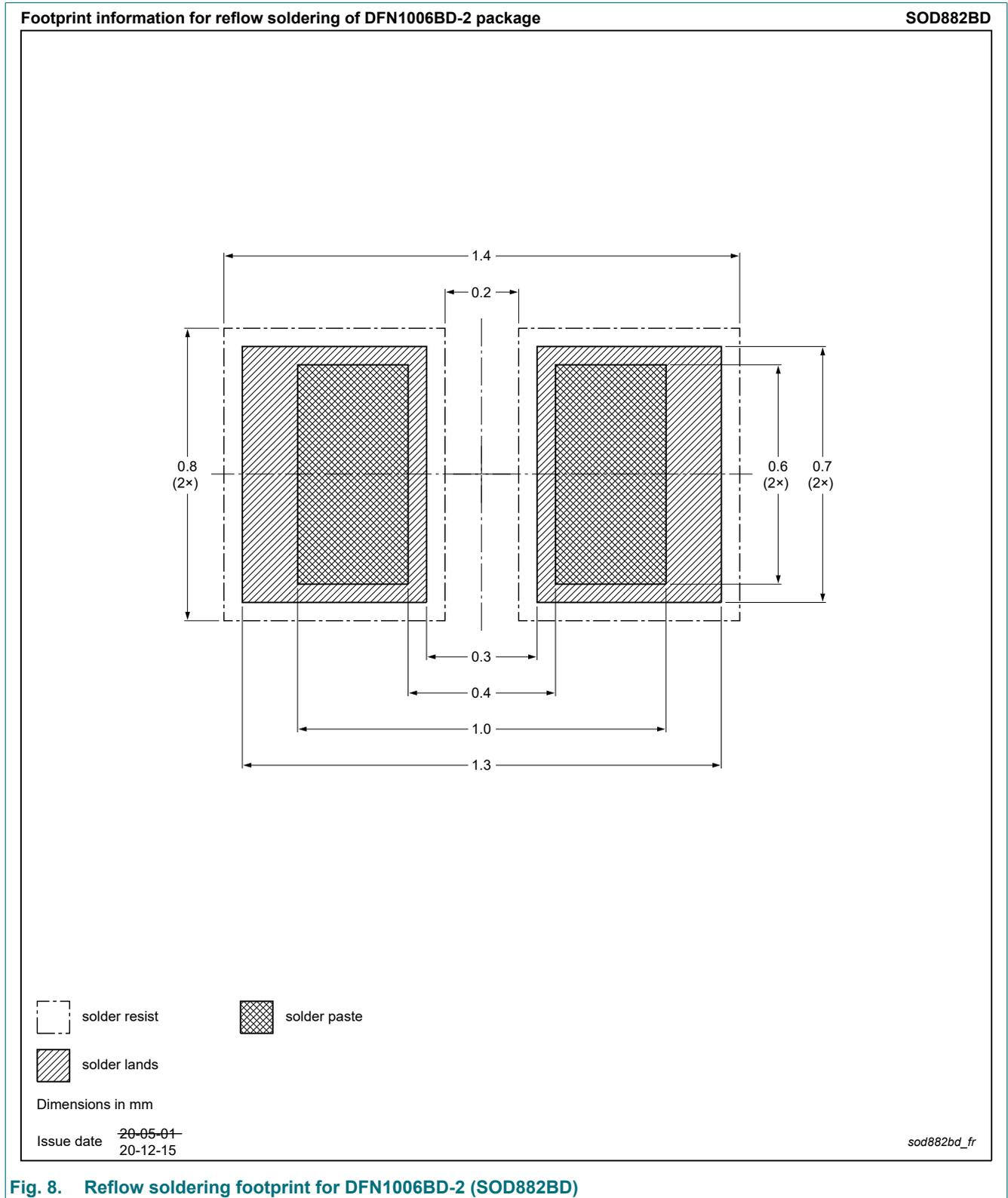
**Fig. 8. Reflow soldering footprint for DFN1006BD-2 (SOD882BD)**
