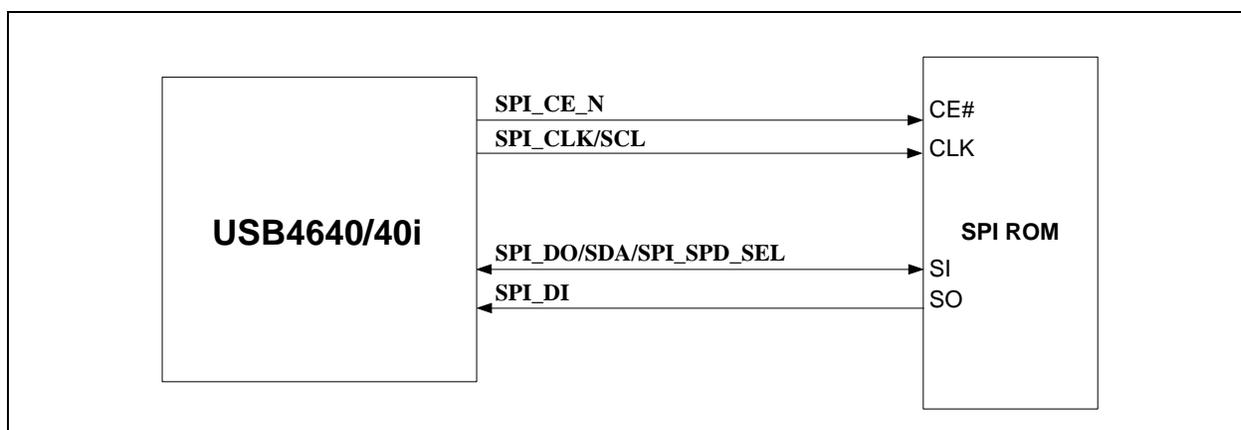
**FIGURE 3-6: I<sup>2</sup>C CONNECTION**
