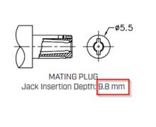
Insertion/extraction force adjusted to 0.3 ~ 2.0 kg
