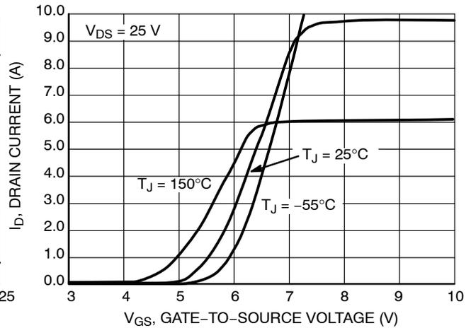
Figure 2. Transfer Characteristics
