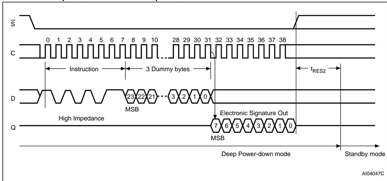
1. The value of the 8-bit electronic signature, for the M25P16, is 14h.
