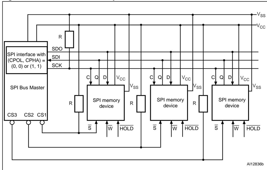
1. The Write Protect ( $\overline{W}$ ) and Hold ( $\overline{HOLD}$ ) signals should be driven, High or Low as appropriate.
