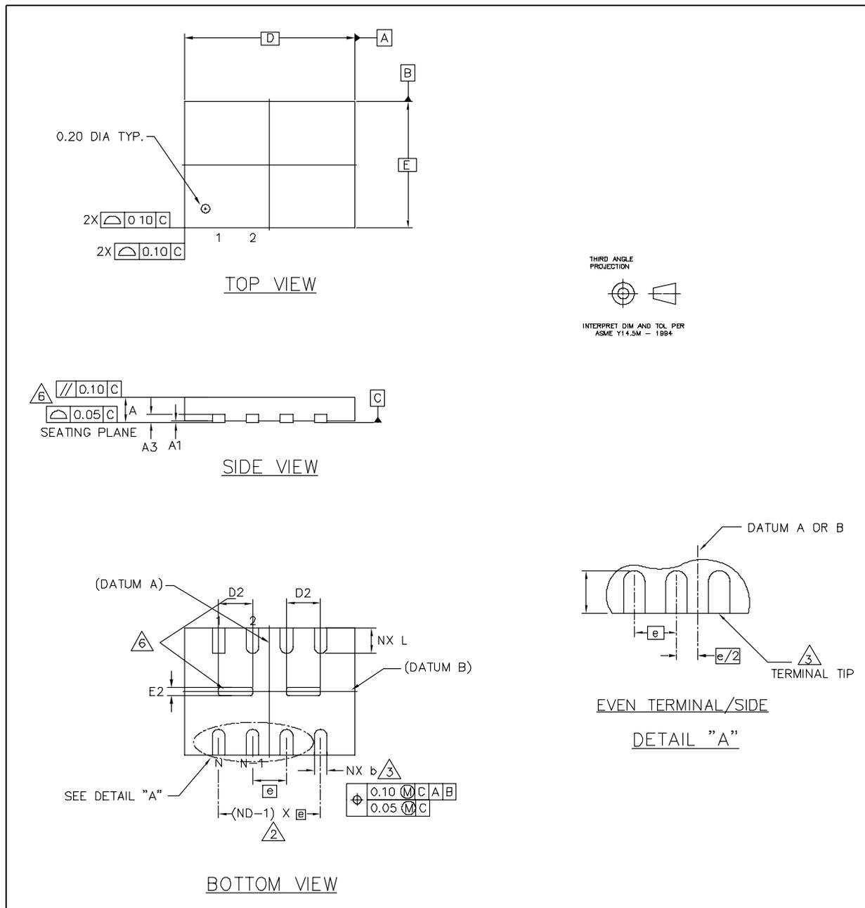
**Table 23. UDFFPN (MLP8) 8-lead ultra thin fine pitch dual flat package no lead, 4X3 mm package mechanical data<sup>(1)</sup>**
