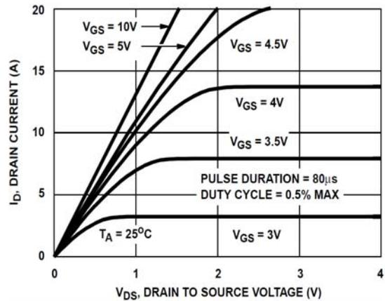
Figure 8. SATURATION CHARACTERISTICS
