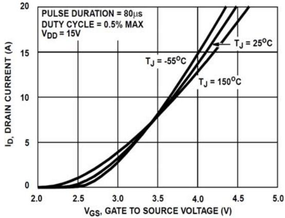
Figure 7. TRANSFER CHARACTERISTICS
