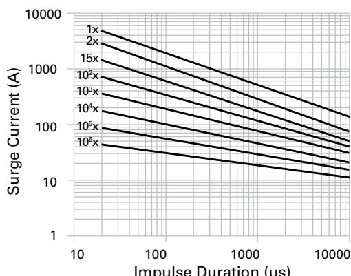
NOTE: If pulse ratings are exceeded, a shift of  $V_{NIDC}$ (at specified current) of more than +/-10% could result. This type of shift, which normally results in a decrease of  $V_{NIDC}$ , may result in the device not meeting the original published specifications, but does not prevent the device from continuing to function, and to provide ample protection.
