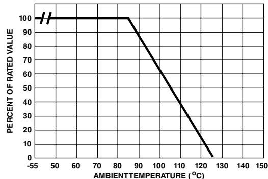
**Figure 1B - Power Derating for Phenolic Coated**
