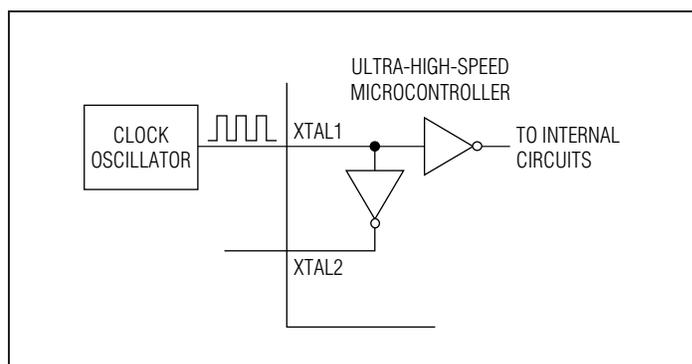
Figure 5-2. Clock Source Input
