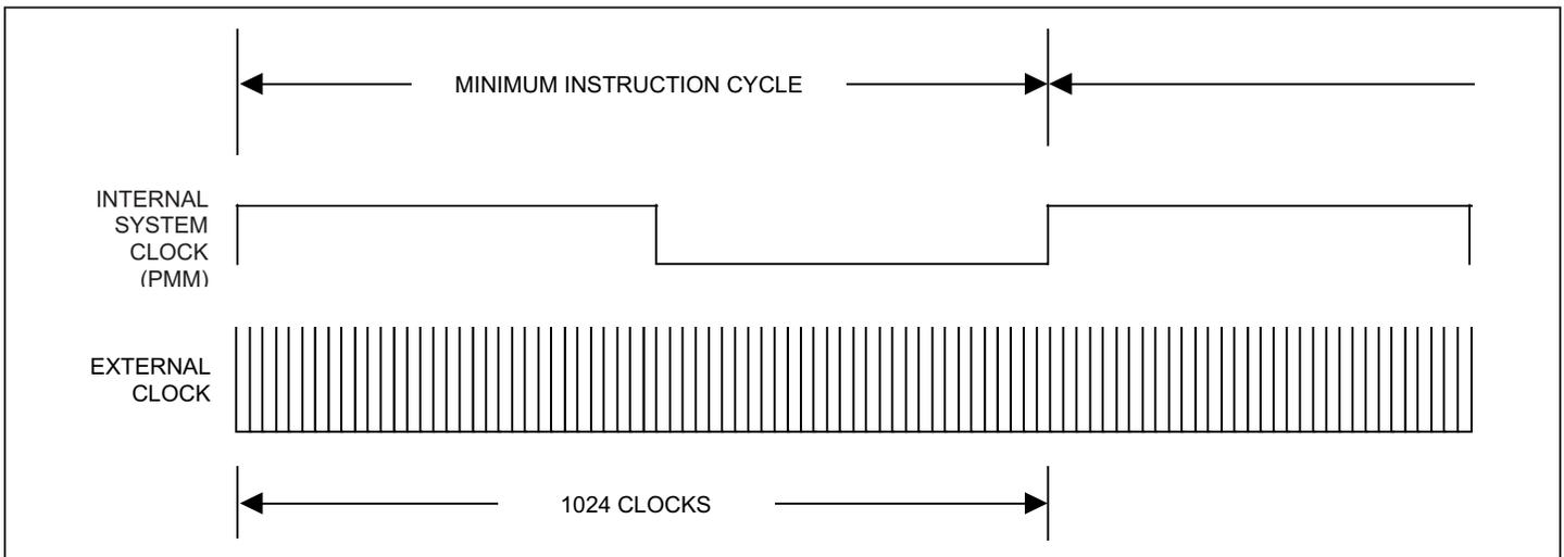
Figure 7-3. Internal Timing Relationships in PMM
