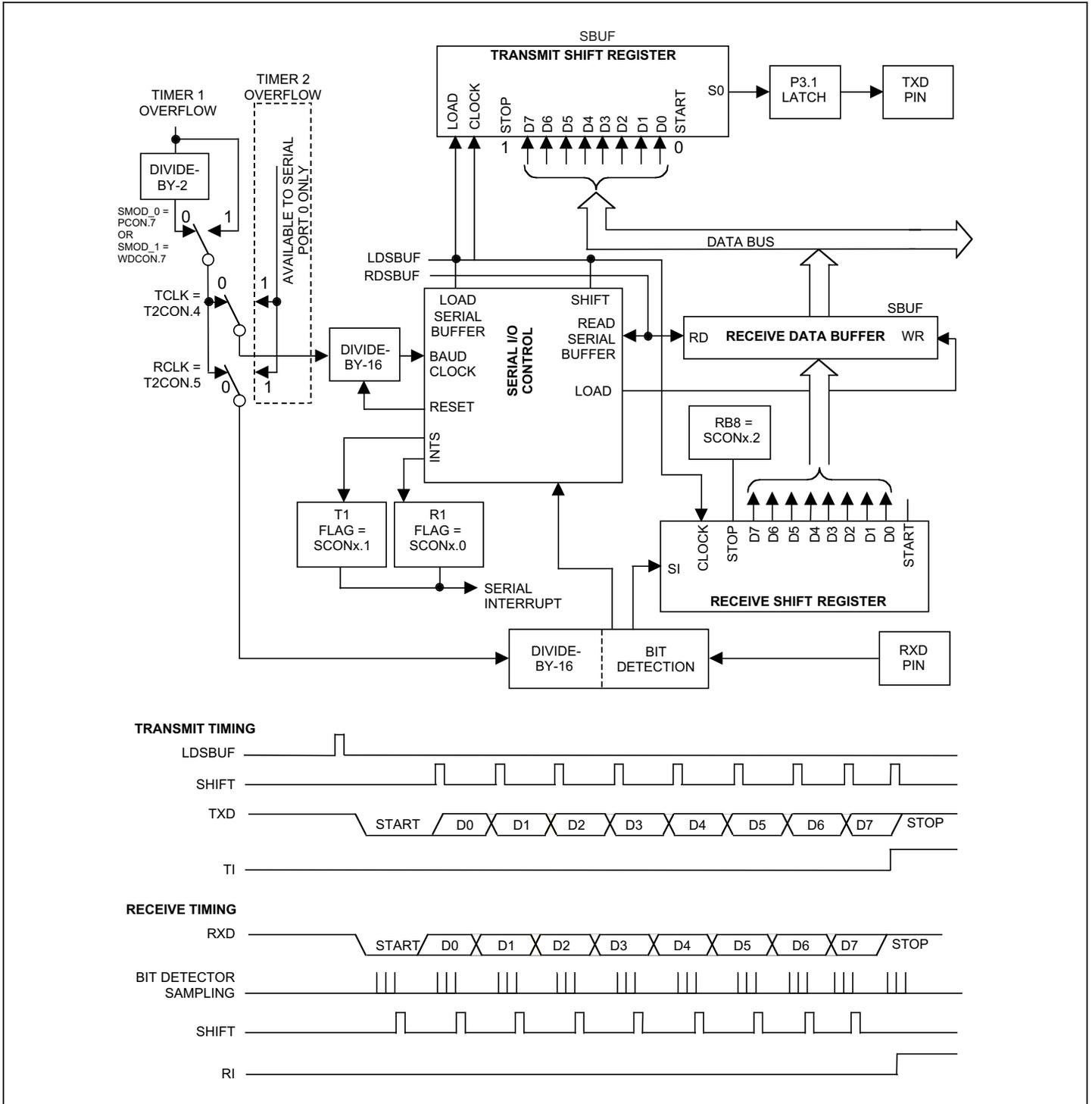
Figure 12-2. Serial Port Mode 1
