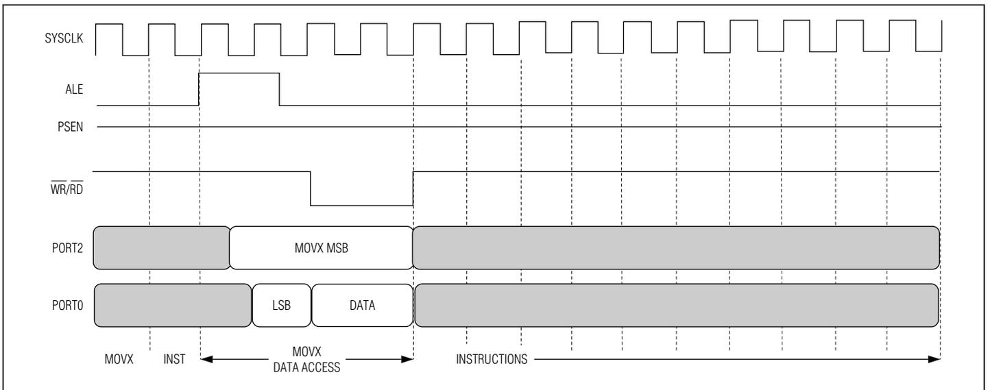
Figure 6-11. Nonpage Mode: MOVX (Two Cycles)
