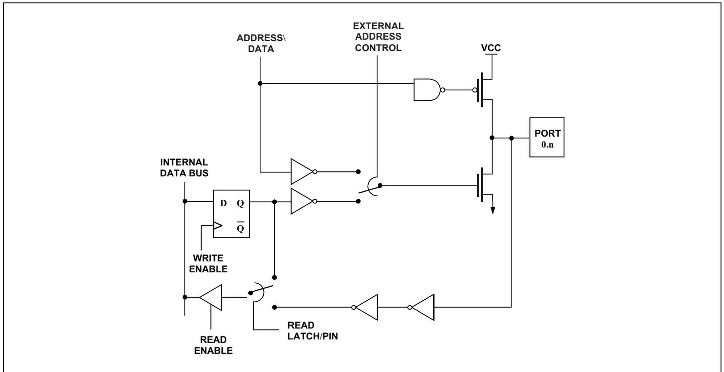
Figure 10-1. Port 0 Functional Circuitry
