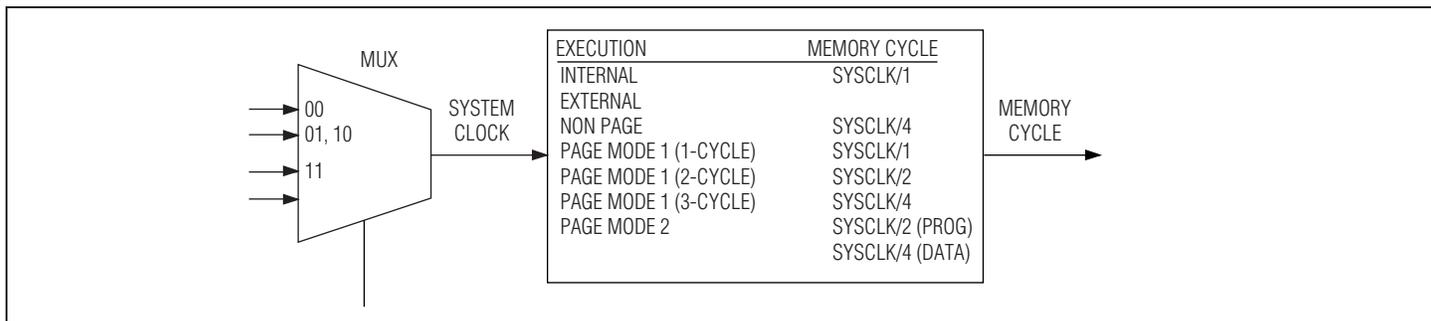
Figure 5-4. Instruction Memory Cycle Determination
