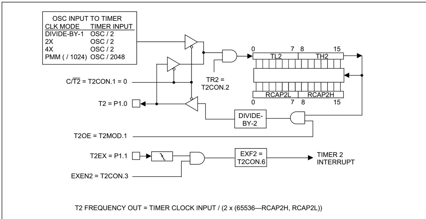
Figure 11-8. Timer/Counter 2 Clock Out Mode Time-Base Selection
