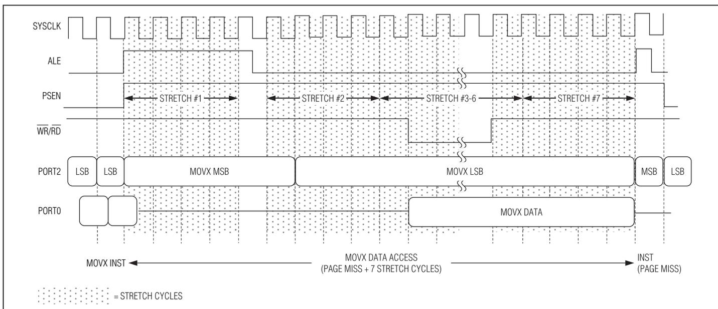
Figure 6-22. One-Cycle Page Mode 1: MOVX (Nine Cycles) External Code Execution
