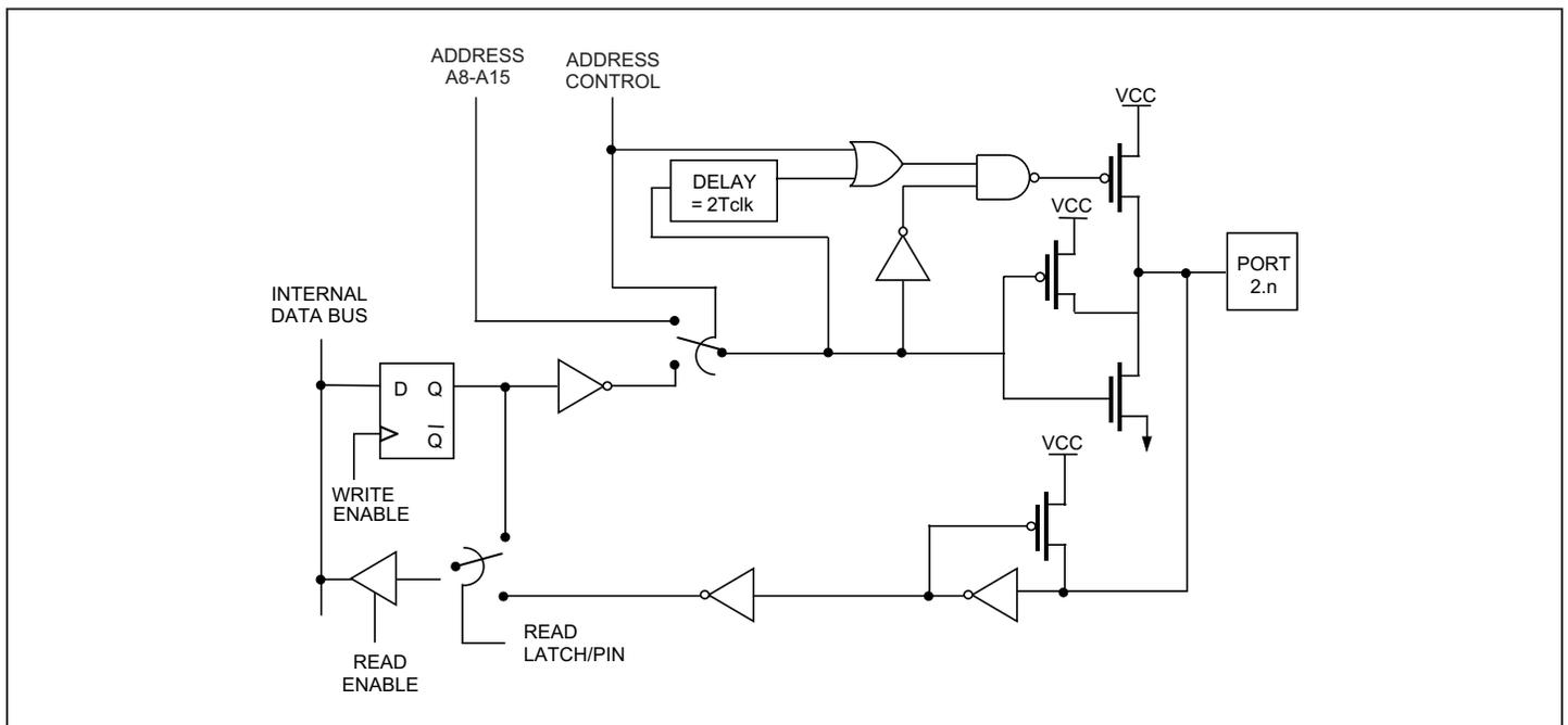
Figure 10-2. Port 2 Functional Circuitry
