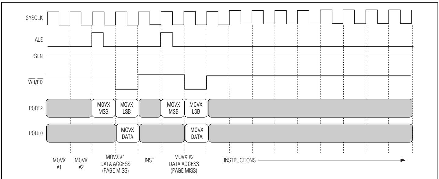
Figure 6-20. One-Cycle Page Mode 1: MOVX (Two Cycles)—MOVX (Two Cycles)
