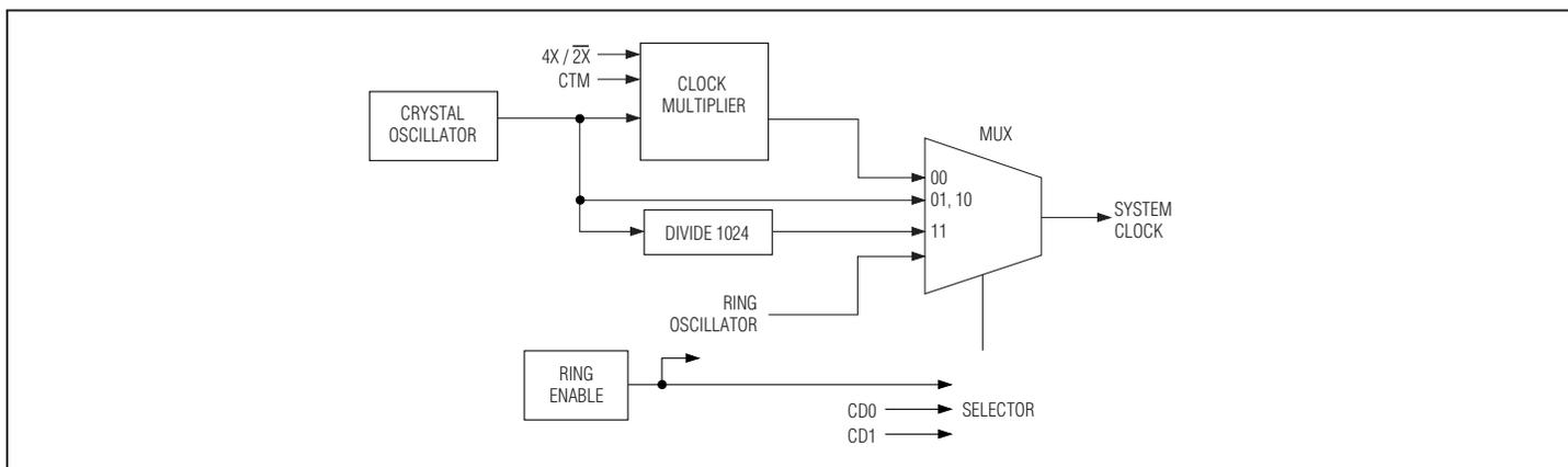
Figure 5-3. System Clock Sources
