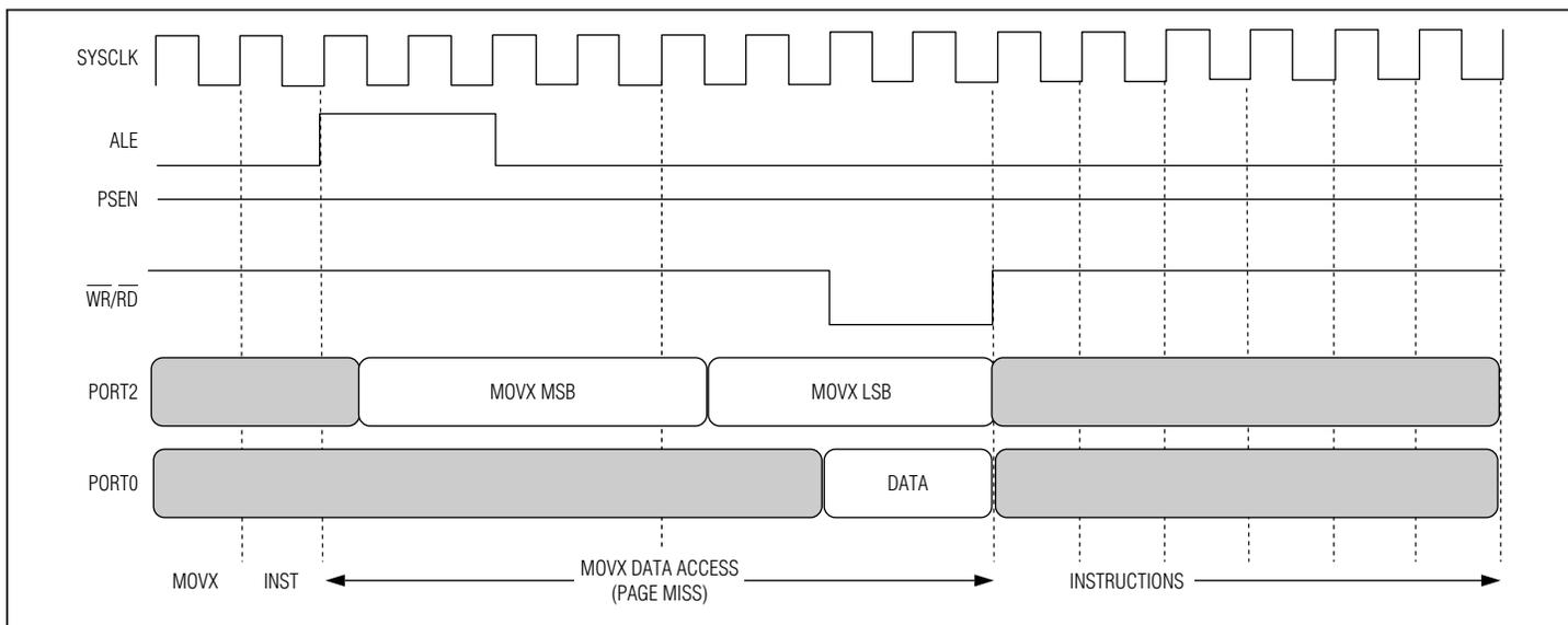
Figure 6-13. Four-Cycle Page Mode 1: MOVX (Two Cycles)
