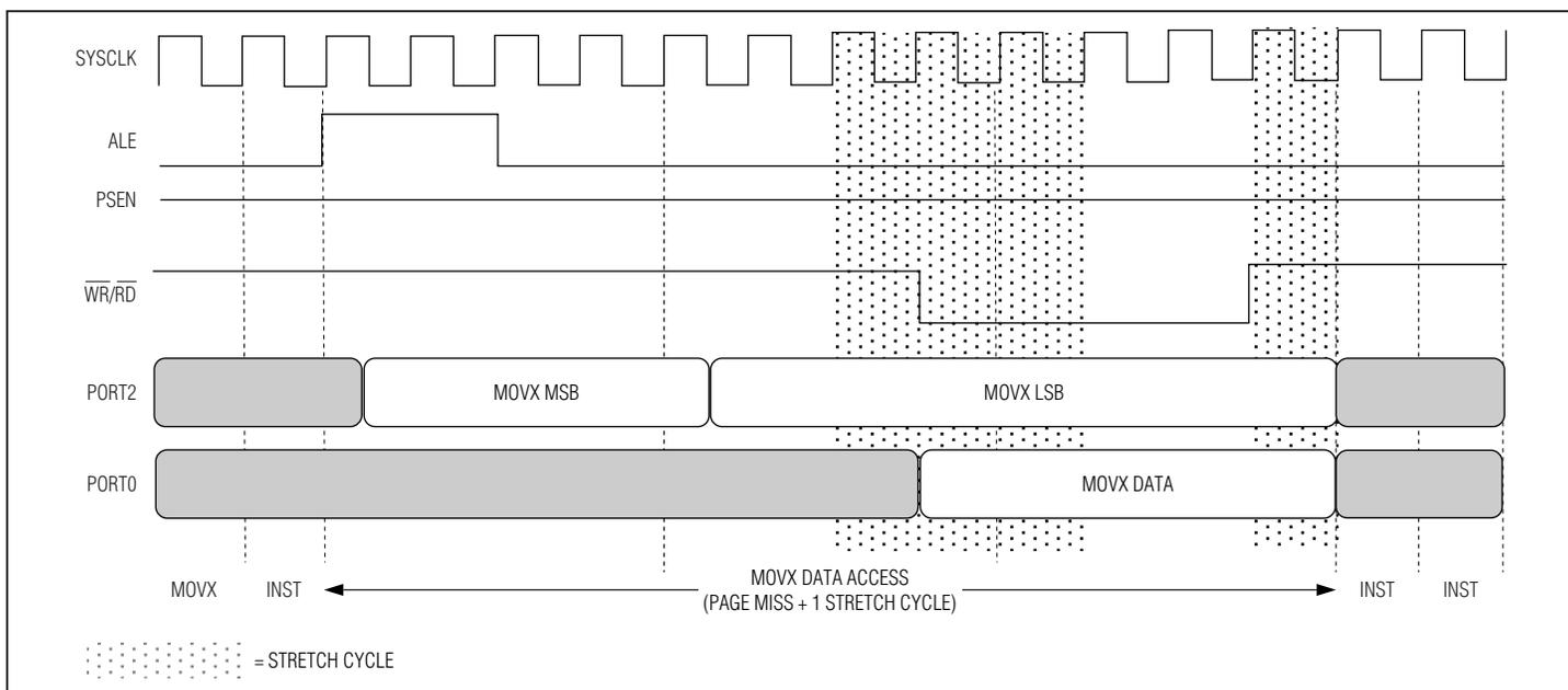
Figure 6-14. Four-Cycle Page Mode 1: MOVX (Three Cycles)
