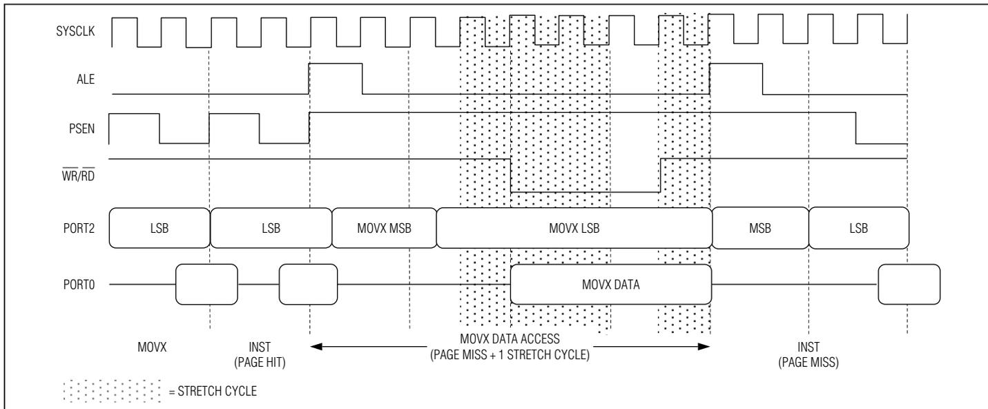
Figure 6-17. Two-Cycle Page Mode 1: MOVX (Three Cycles) External Code Execution with Page Misses
