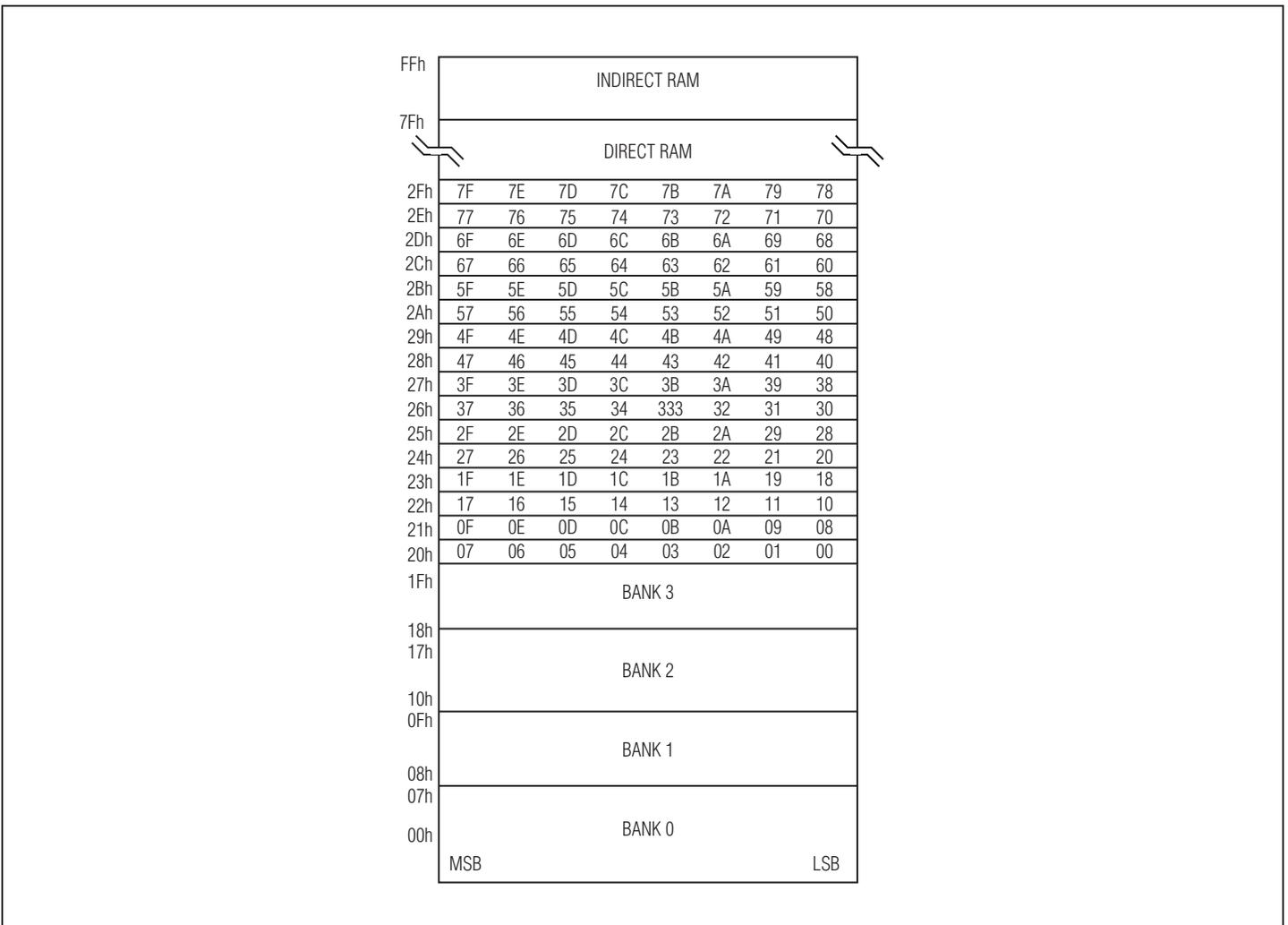
Figure 4-3. Scratchpad Register Addressing
