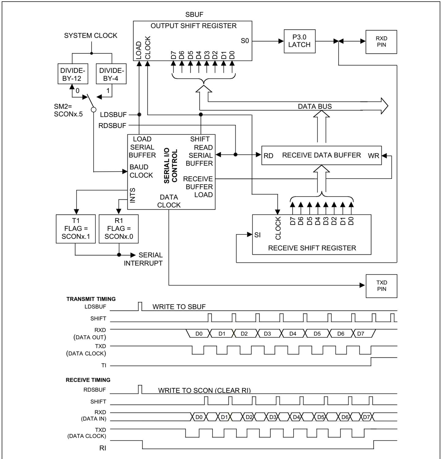
Figure 12-1. Serial Port Mode 0
