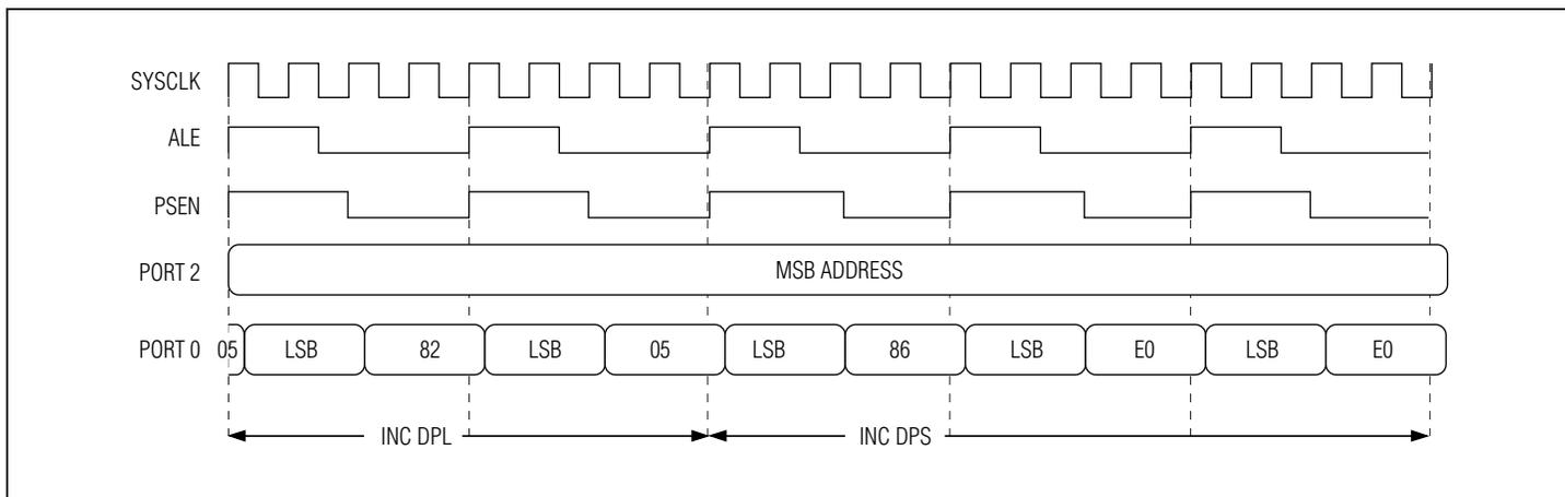
Figure 5-6. Nonpage Mode: INC Direct (Two Cycles) – INC Direct (Three Cycles)
