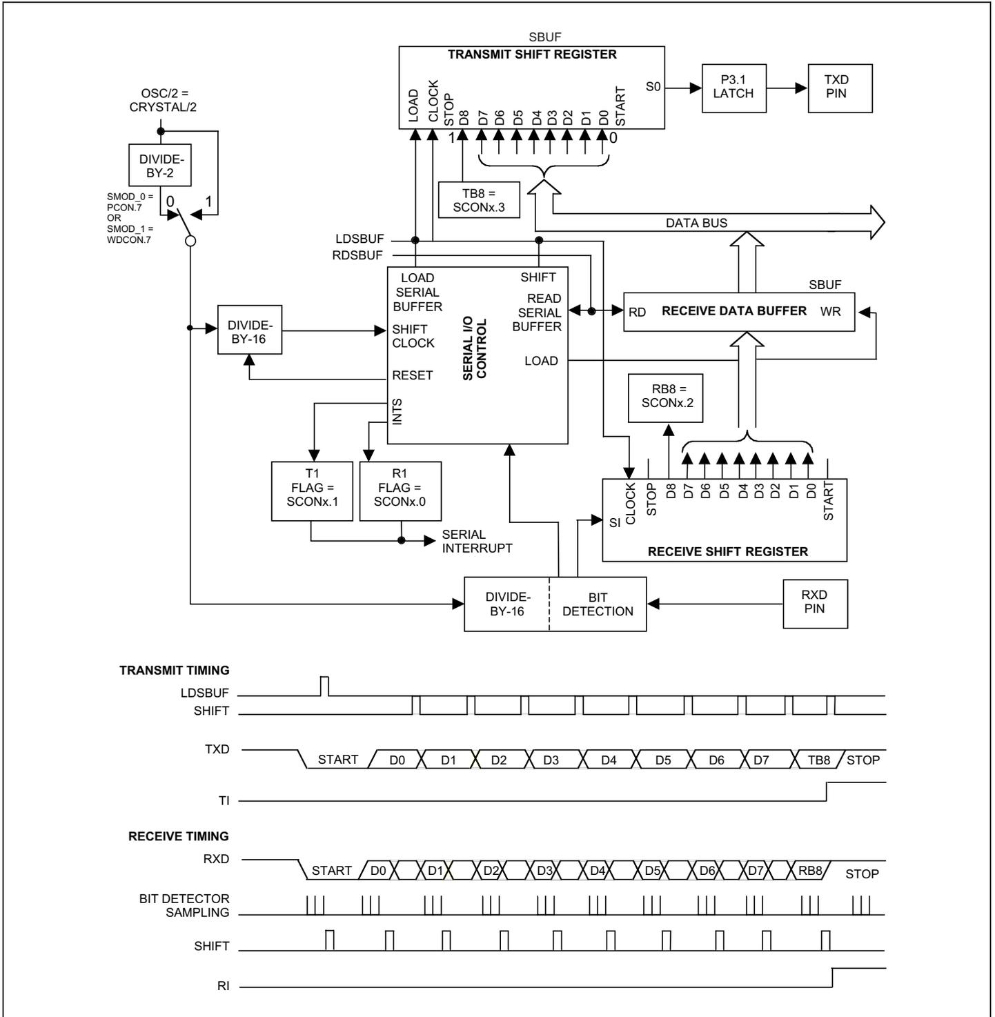
Figure 12-3. Serial Port Mode 2
