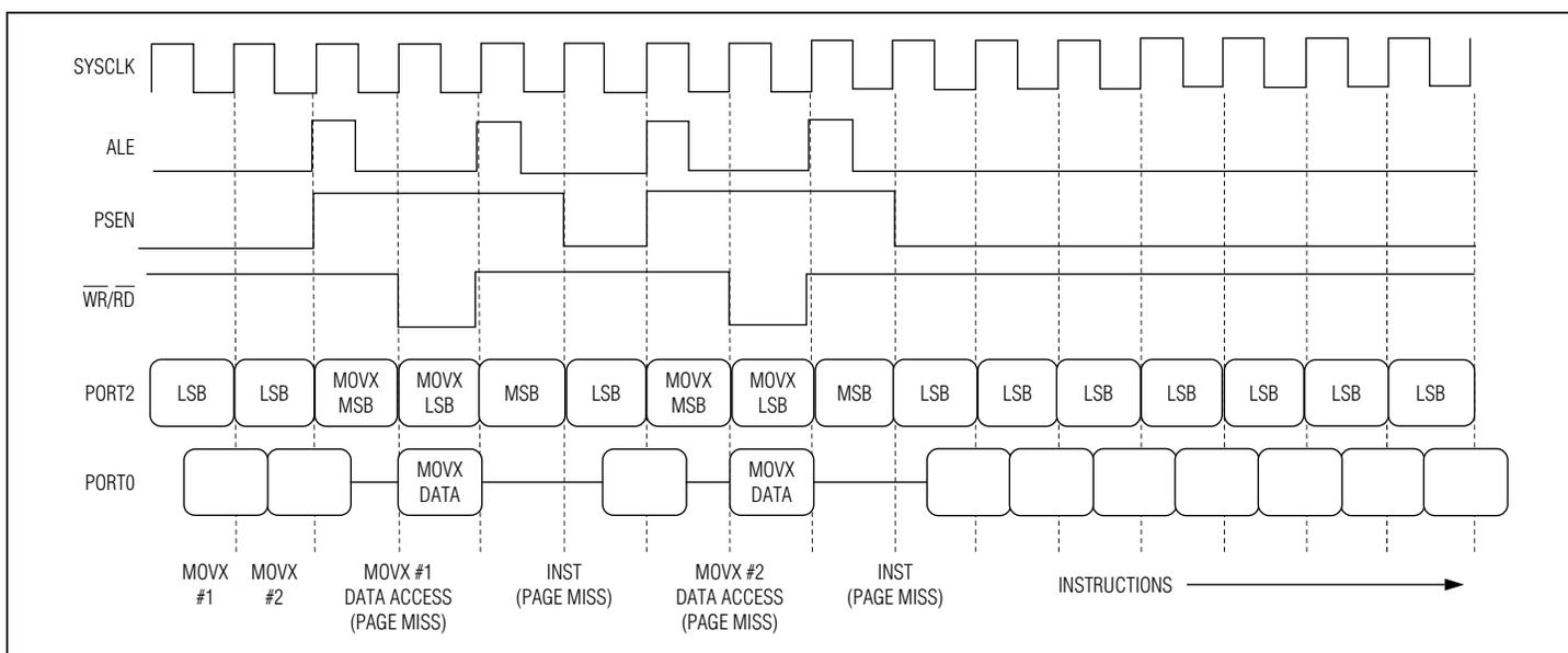
Figure 6-21. One-Cycle Page Mode 1: MOVX (Two Cycles)—MOVX (Two Cycles) External Code Execution
