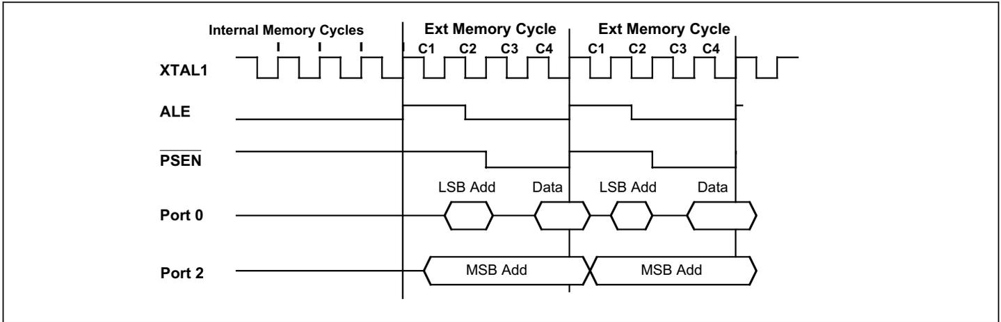
Figure 10-3. External Program Memory Access (Nonpage Model)
