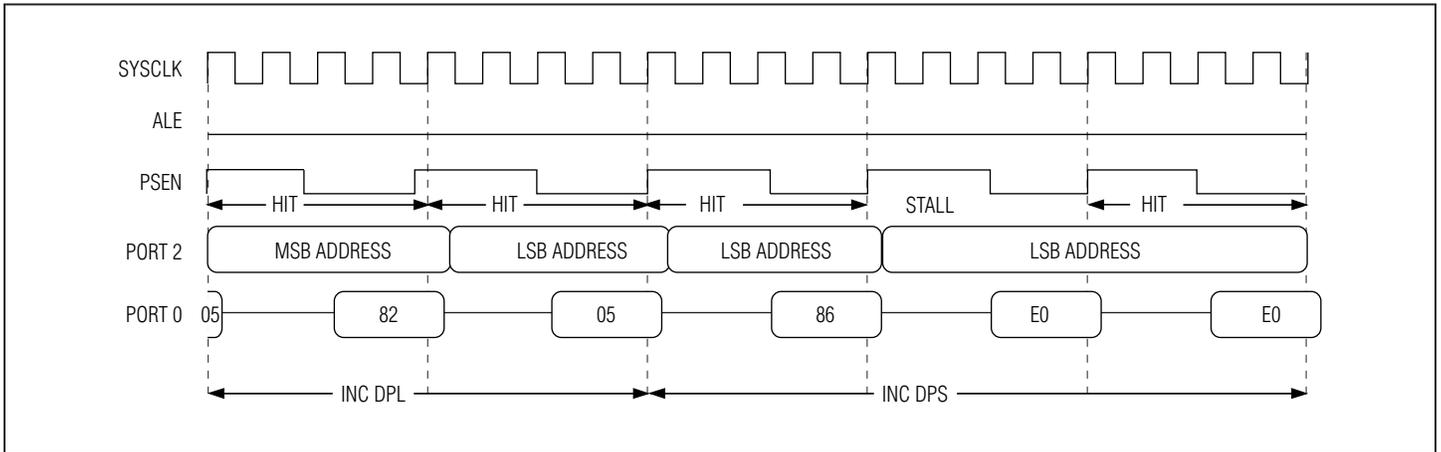
Figure 5-11. Four-Cycle Page Mode 1: INC Direct (Two Cycles) – INC Direct (Three Cycles)
