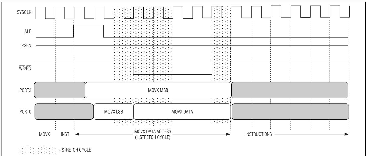
Figure 6-12. Nonpage Mode: MOVX (Three Cycles)
