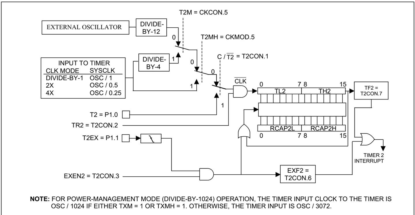
Figure 11-5. Timer/Counter 2 Autoreload Mode (CP/RL2 = 0, DCEN = 0)
