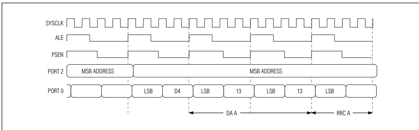
Figure 5-5. Nonpage Mode: DA A – RRC A
