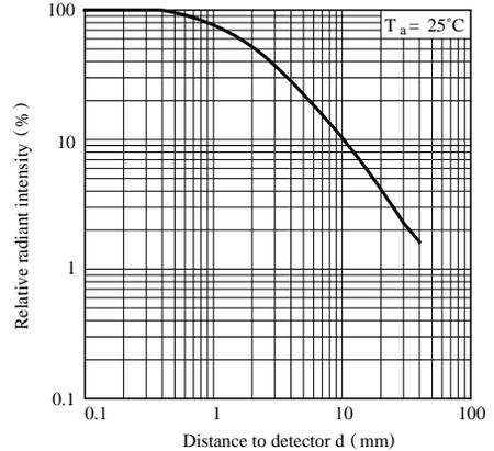
**Fig. 9 Relative Collector Current vs. Distance (Detector : PT480)**
