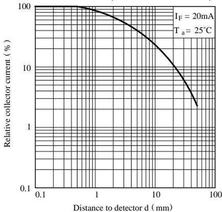
**Fig.10 Radiation Diagram (GL480Q/GL483Q)**
