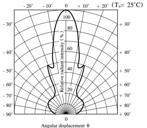
**Fig.11 Radiation Diagram (GL480) (Ta = 25°C)**
