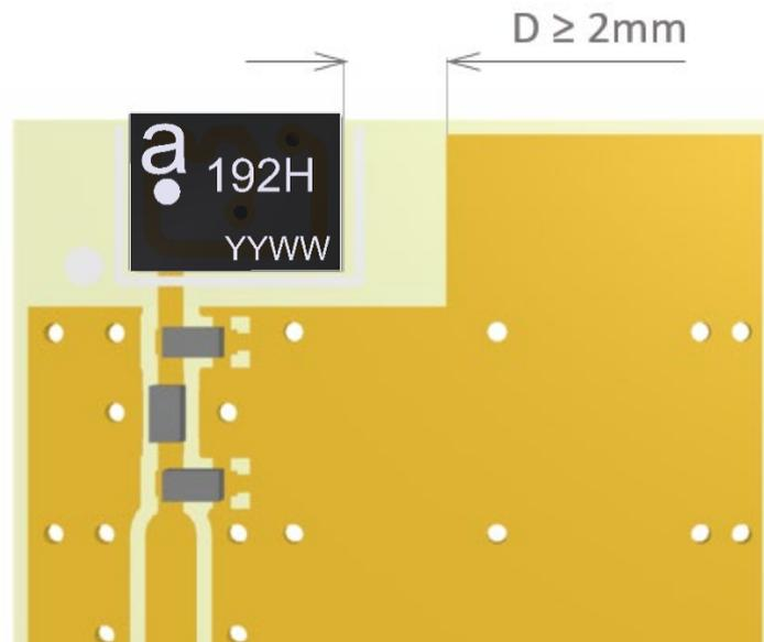
Additional ground and components near the antenna should be at a distance of at least 2 mm. Where possible the antenna should be clear of ground from both sides, although the antenna can work well with a minimum clearance of  $D \geq 2$  mm as shown in the drawing above.
