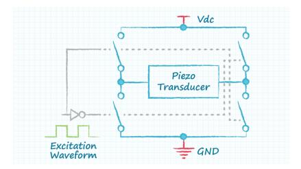
A full bridge circuit is often used for driving piezo transducers. The advantage of using the full bridge comprised of four switches is the peak-to-peak voltage applied across the transducer is twice as large as the available supply voltage. The use of a full bridge driver will cause a resultant increase in the sound volume of about 6 dB due to the doubling of the voltage applied to the transducer.
