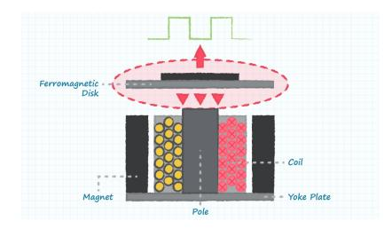
Figure 1: Construction of a typical magnetic buzzer
