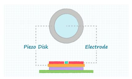
Figure 2: Construction of a typical piezo buzzer
