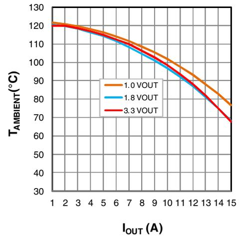
Figure 20: Maximum  $T_{AMBIENT}$  vs  $I_{OUT}$ ,  $V_{IN}=5V$
