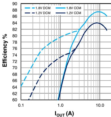
Figure 23: Efficiency,  $V_{IN}=19.6V$
