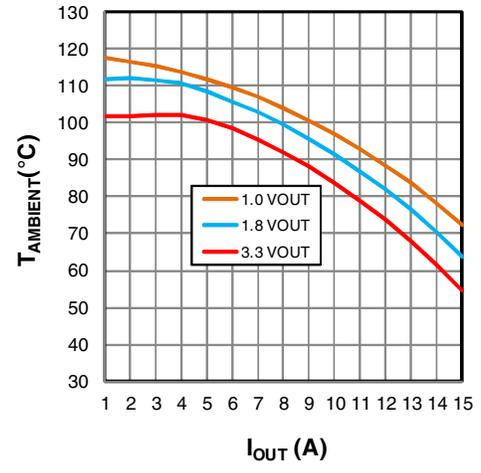
Figure 22: Maximum  $T_{AMBIENT}$  vs  $I_{OUT}$ ,  $V_{IN}=12V$
