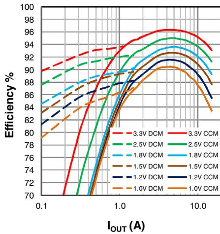
Figure 19: Efficiency,  $V_{IN}=5V$
