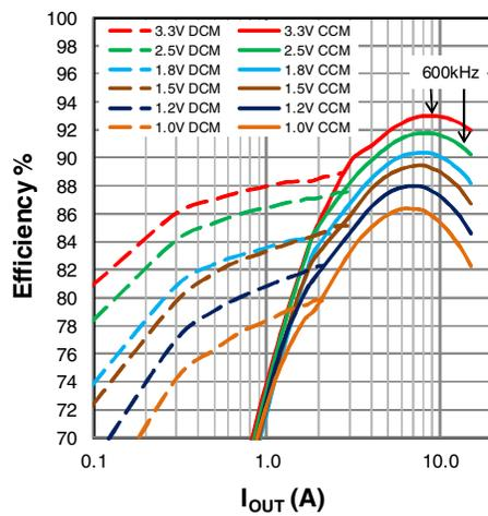
Figure 21: Efficiency,  $V_{IN}=12V$
