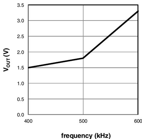
Figure 12: Maximum recommended  $V_{OUT}$  versus  $f$ ,  $V_{IN}=12V$
