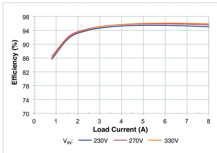
Figure 9 — Efficiency at  $T_{CASE} = 85^{\circ}C$
