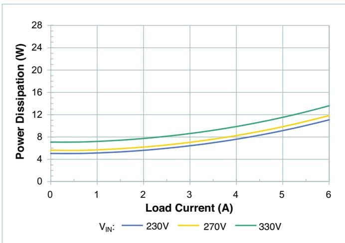
Figure 12 — Power dissipation at  $T_{CASE} = 100^{\circ}C$
