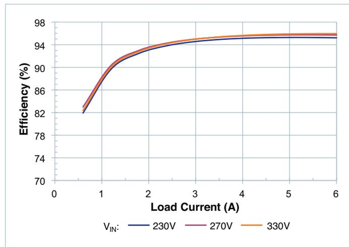
Figure 11 — Efficiency at  $T_{CASE} = 100^{\circ}C$
