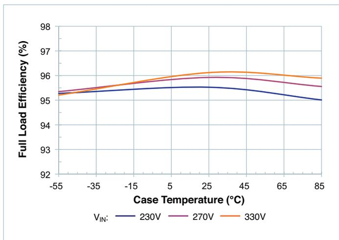
Figure 4 — Full load efficiency vs.  $T_{MAX}$  restricted
