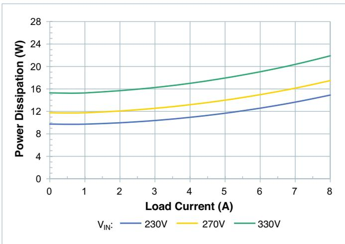
Figure 6 — Power dissipation at  $T_{CASE} = -55^{\circ}C$
