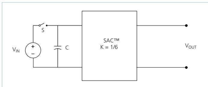
**Figure 22** — Sine Amplitude Converter™ with input capacitor
