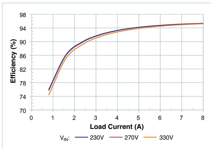
Figure 5 — Efficiency at  $T_{CASE} = -55^{\circ}C$
