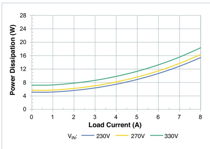
Figure 10 — Power dissipation at  $T_{CASE} = 85^{\circ}C$
