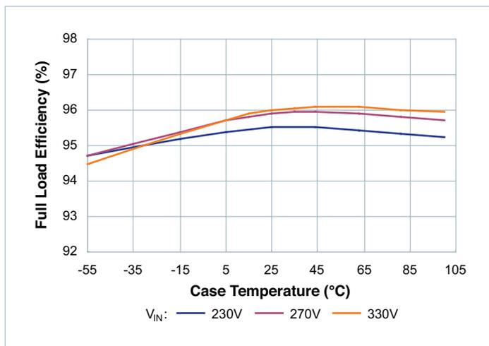
Figure 3 — Full load efficiency vs. full  $T_{MAX}$  range
