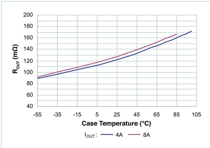
Figure 13 —  $R_{OUT}$  vs. temperature; nominal input
