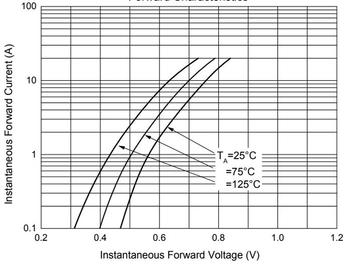
Fig. 4 - MBR30150CTH Typical Instantaneous Forward Characteristics
