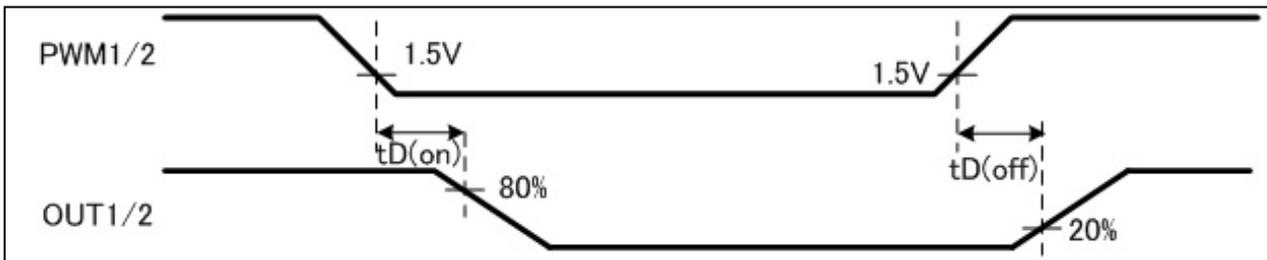
Figure 10.2. Driver output delay time
