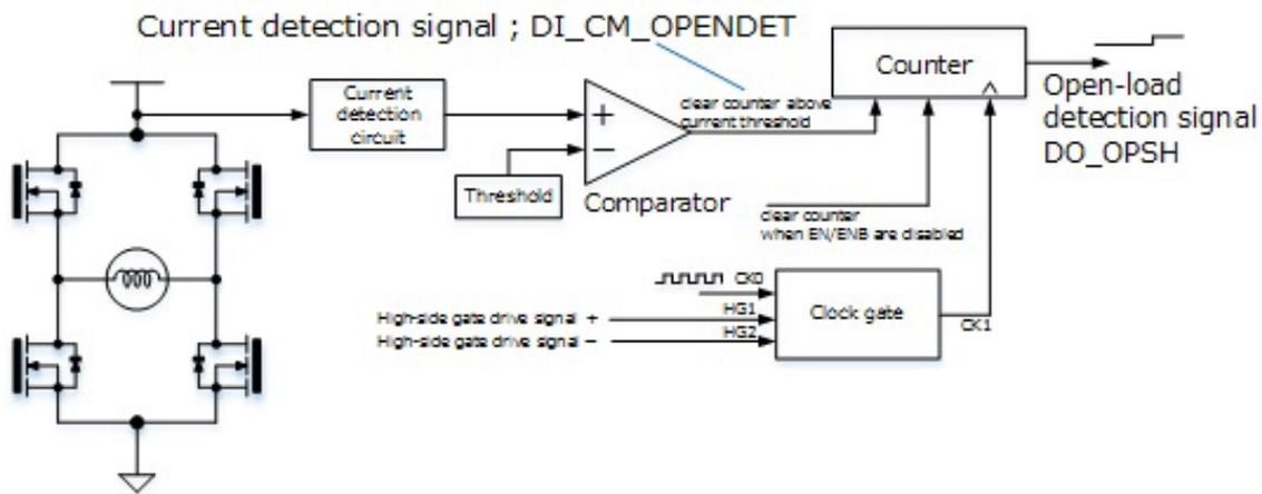
**Figure 7.22 Open-load detection during operation: block diagram**
