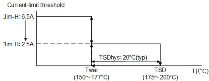
**Figure 7.17 Temperature-adjusted current-limit control**
