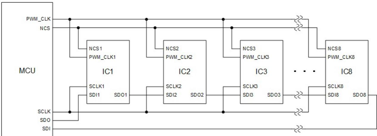
**Figure 7.28 Example SPI daisy-chain connection (eight connected ICs)**
