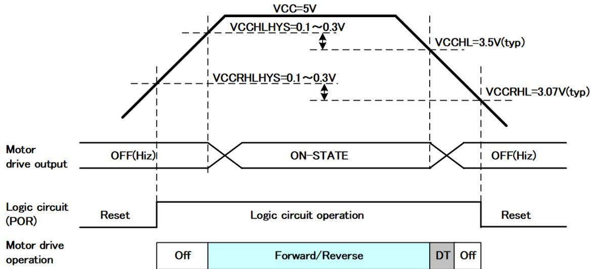
Figure 7.37 VCC under-voltage detection and POR threshold characteristics
