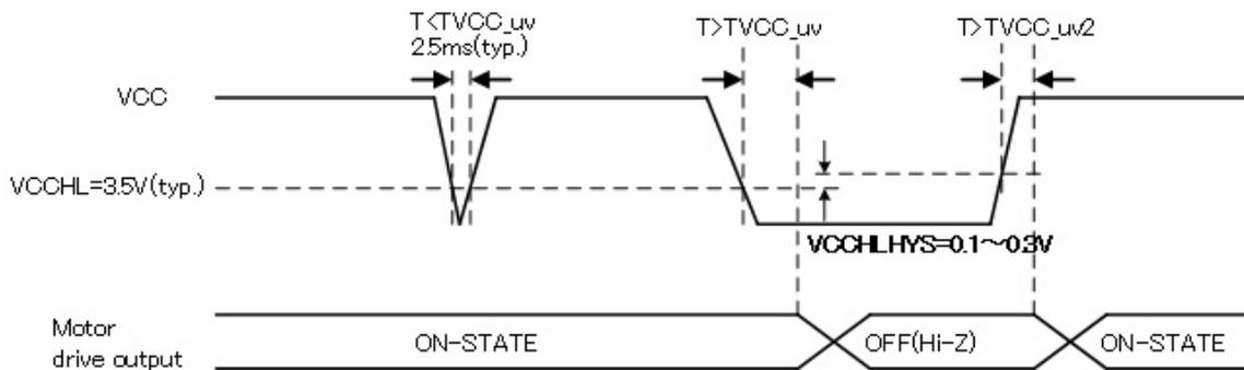
Figure 7.38 VCC under-voltage detection timing chart 1
