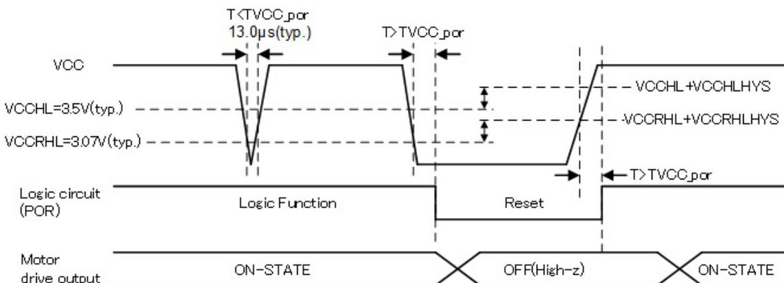
Figure 7.39 VCC under-voltage POR timing chart 1
