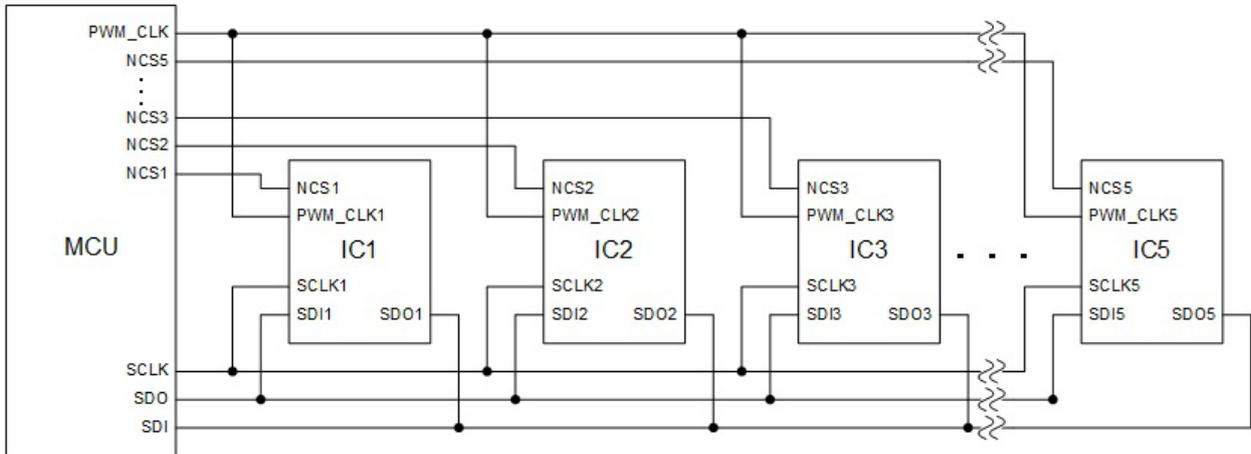
**Figure 7.27 Example SPI parallel connection (five connected ICs)**
