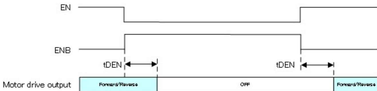
**Figure 7.1. EN/ENB signals and motor drive output**
