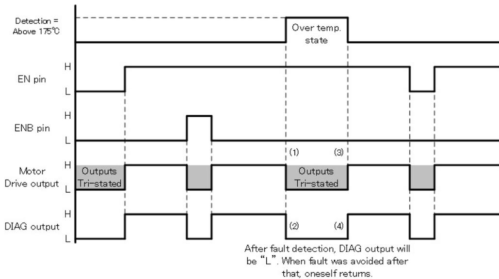
**Figure 7.40 Over-temperature detection timing chart**
