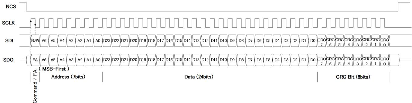
**Figure 7.26 SPI communication format**
