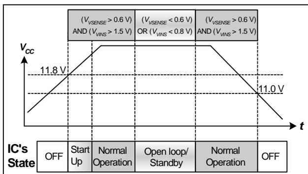
Figure 3 State of Operation respect to VCC
