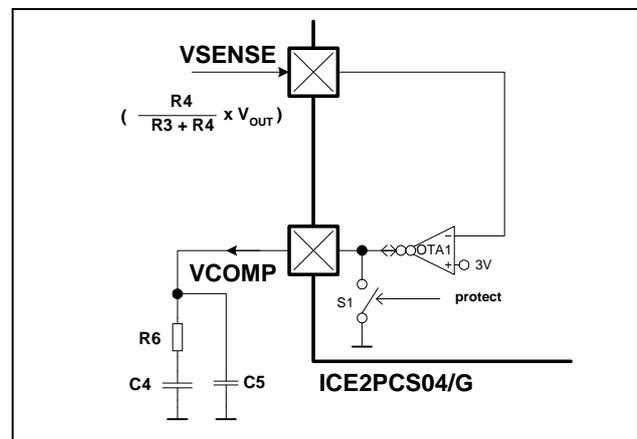
Figure 4 Startup Circuit
