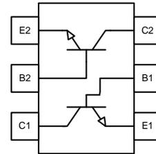
Figure 2. Internal Connection
