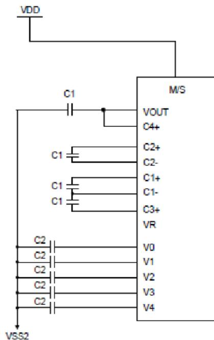
C1: 1uF-4.7uF for Voltage rating from 10-35V
