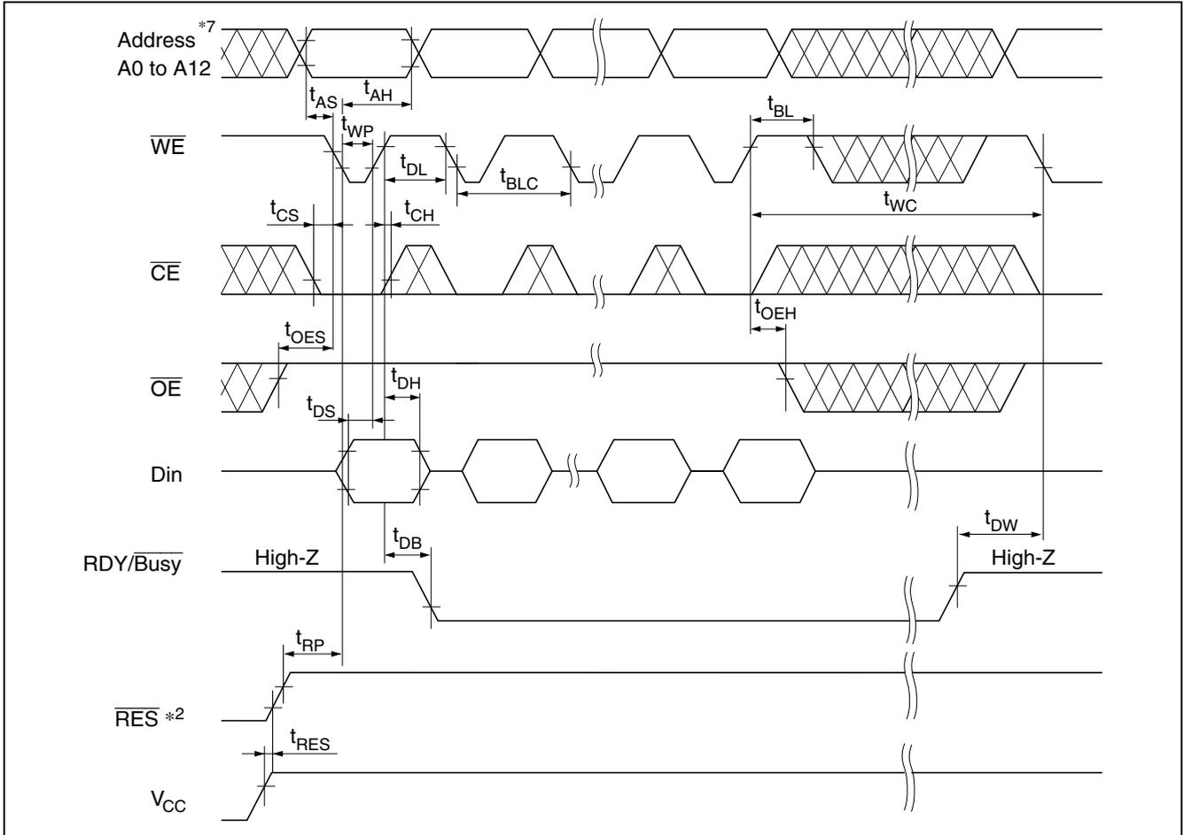
Page Write Timing Waveform(2) ( $\overline{\text{CE}}$  Controlled)
