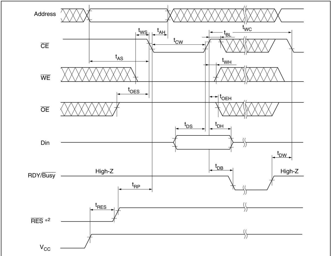
Page Write Timing Waveform(1) ( $\overline{WE}$  Controlled)
