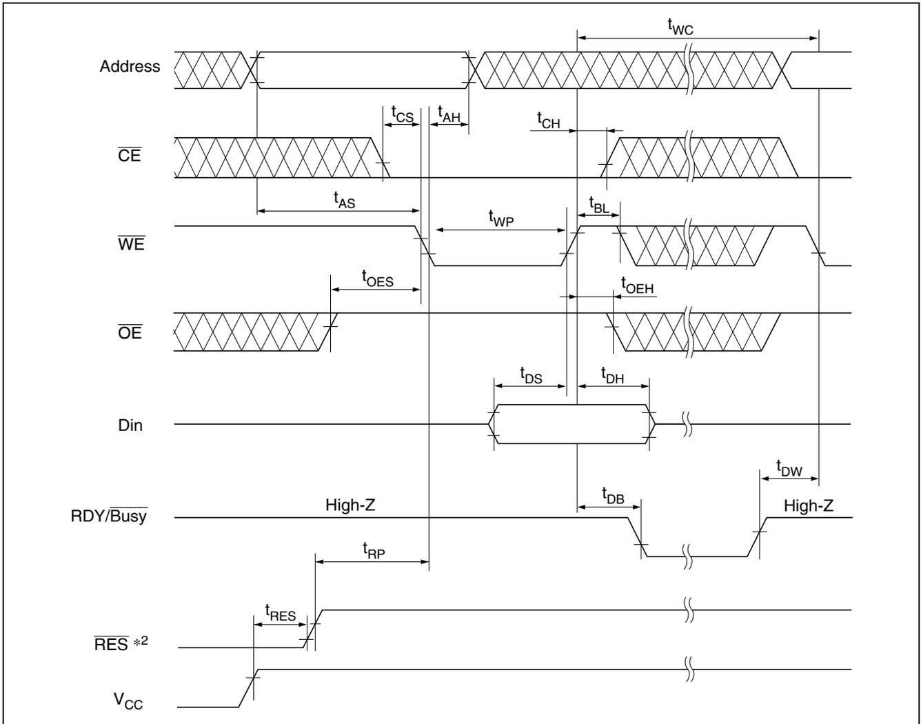
**Byte Write Timing Waveform(2) ( $\overline{CE}$  Controlled)**
