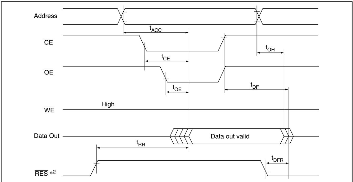
**Byte Write Timing Waveform(1) ( $\overline{WE}$  Controlled)**
