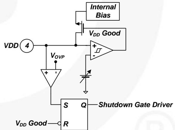
Figure 21. Internal OVP Block
