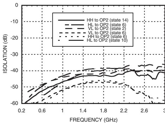
**Isolation When HH is Connected to OP2\***
