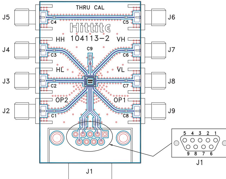
The circuit board used in the final application should be generated with proper RF circuit design techniques. Signal lines at the RF port should have 50 ohm impedance and the package ground leads and exposed paddle should be connected directly to the ground plane similar to that shown above. A generous number of ground vias should be used to interconnect top/bottom ground planes. The evaluation circuit board shown above is available from Hittite Microwave Corporation upon request.
