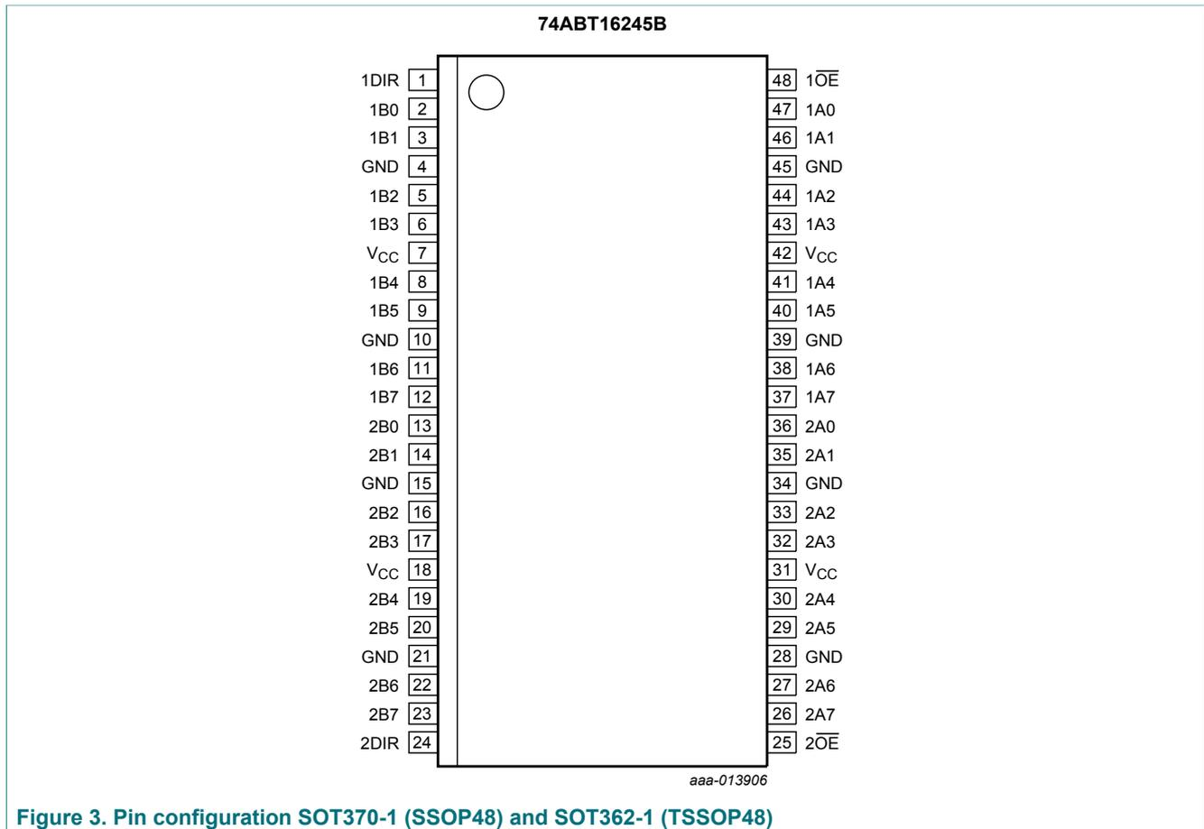
Figure 3. Pin configuration SOT370-1 (SSOP48) and SOT362-1 (TSSOP48)
