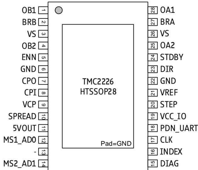
Figure 2.1 TMC2226 Pinning Top View – type: HTSSOP 28, 9.7x6.4mm<sup>2</sup> over pins, 0.65mm pitch
