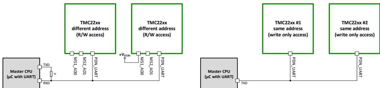
Figure 4.1 Attaching the TMC2226 to a microcontroller UART
