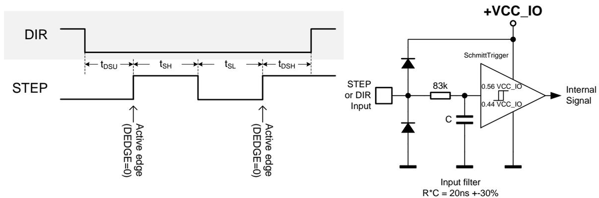
Figure 13.1 STEP and DIR timing, Input pin filter
