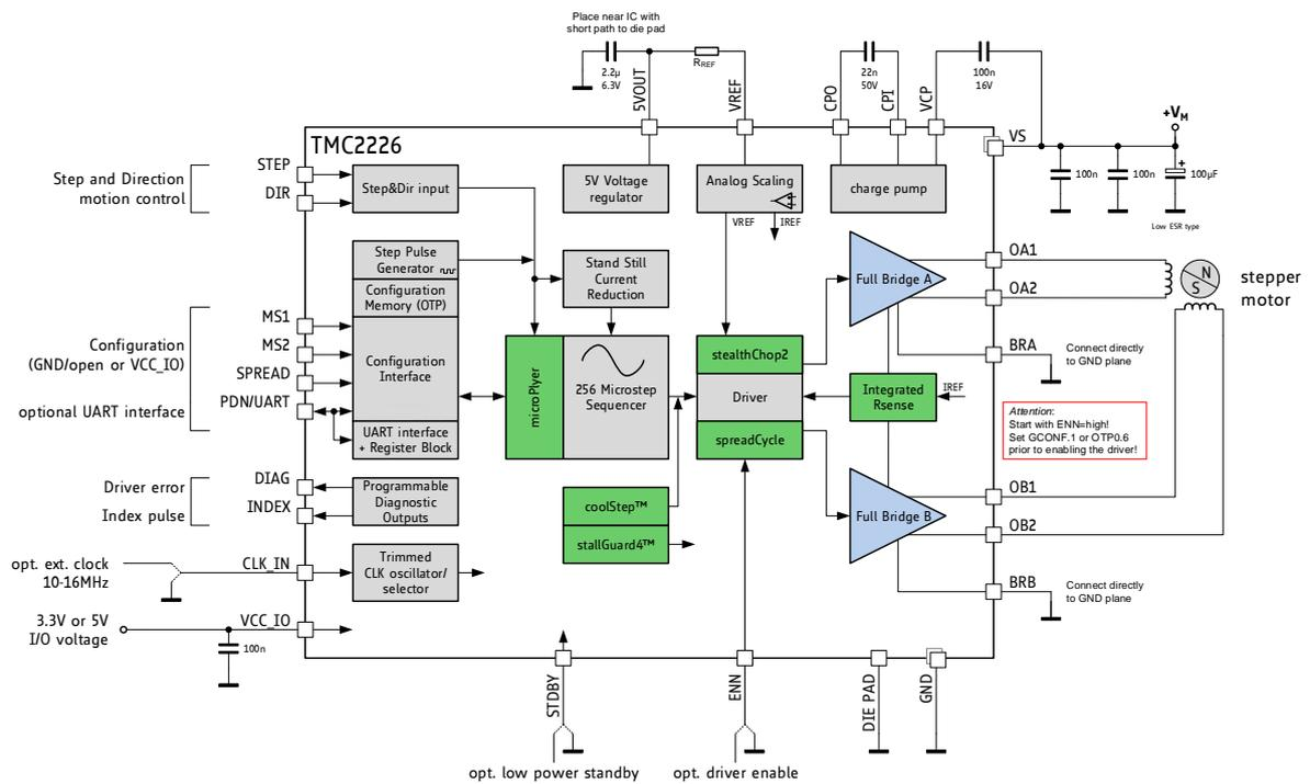
Figure 3.2 Application circuit using RDSon based sensing
