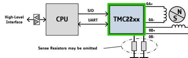
A CPU operates the driver via step and direction signals. It accesses diagnostic information and configures the TMC2226 via the UART interface. The CPU manages motion control and the TMC2226 drives the motor and smoothens and optimizes drive performance.
