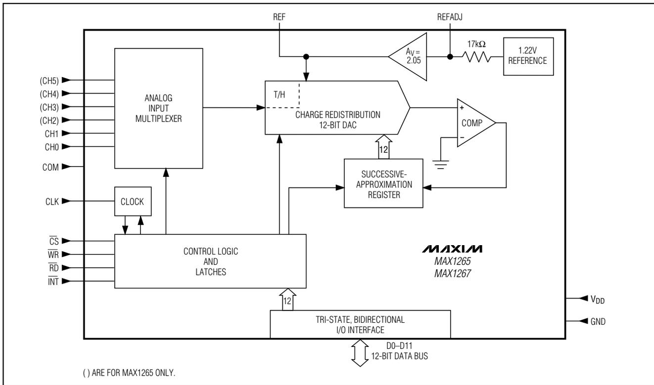
Figure 2. Simplified Functional Diagram of 6-/2-Channel MAX1265/MAX1267
