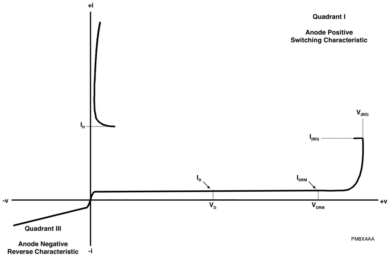
**Figure 1. Voltage-Current Characteristic for A and K Terminals**
