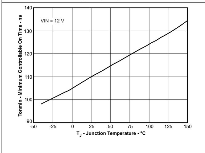
Figure 5. Minimum Controllable on Time vs Junction Temperature
