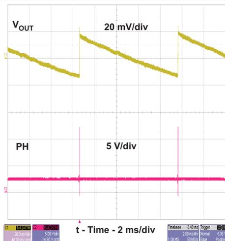
Figure 22. TPS54332 Output Ripple during Eco-Mode Operation
