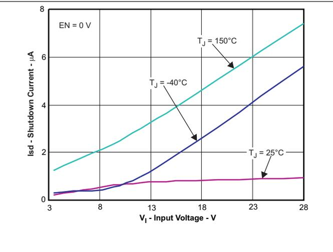
Figure 2. Shutdown Quiescent Current vs Input Voltage
