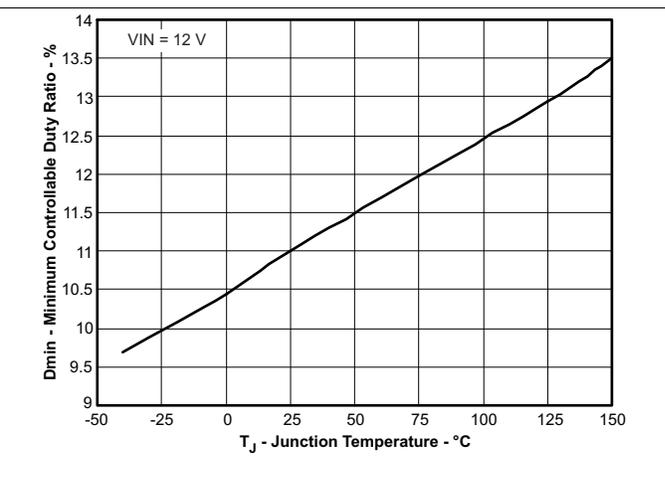
Figure 6. Minimum Controllable Duty Ratio vs Junction Temperature
