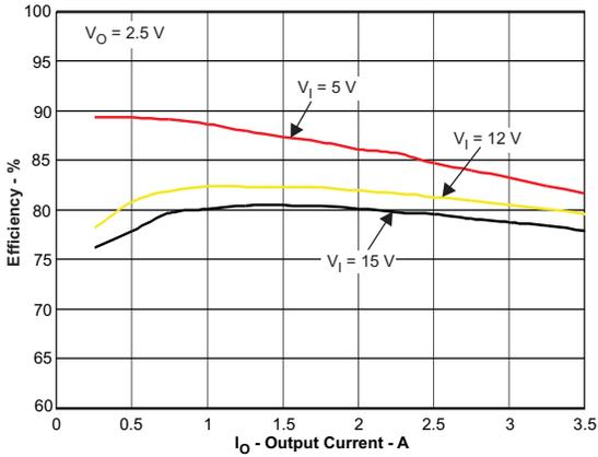
Figure 13. TPS54332 Efficiency
