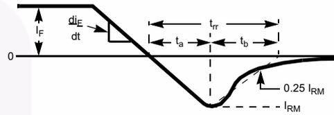
Figure 13.  $t_{rr}$  Waveforms and Definitions
