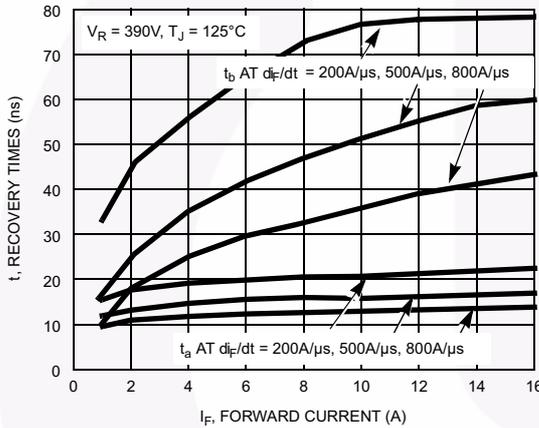
Figure 3.  $t_a$  and  $t_b$  Curves vs Forward Current
