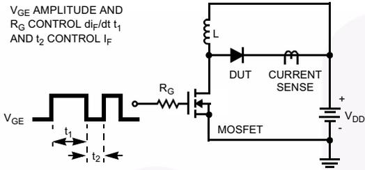
Figure 12.  $t_{rr}$  Test Circuit
