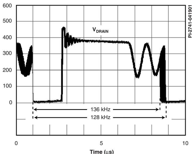
Figure 4. Frequency Jitter.
