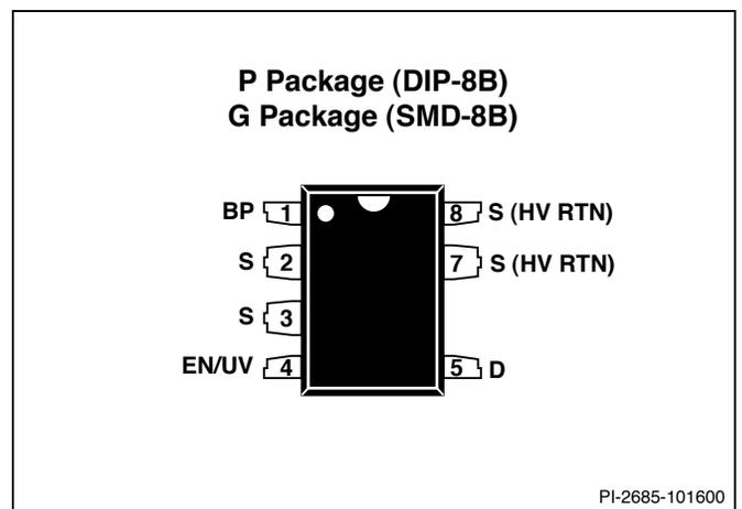
Figure 3. Pin Configuration.
