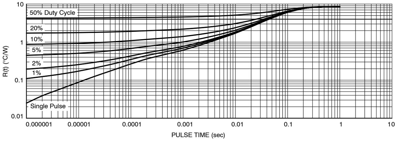
Figure 13. Thermal Characteristics
