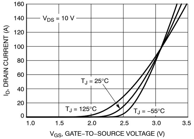
Figure 2. Transfer Characteristics
