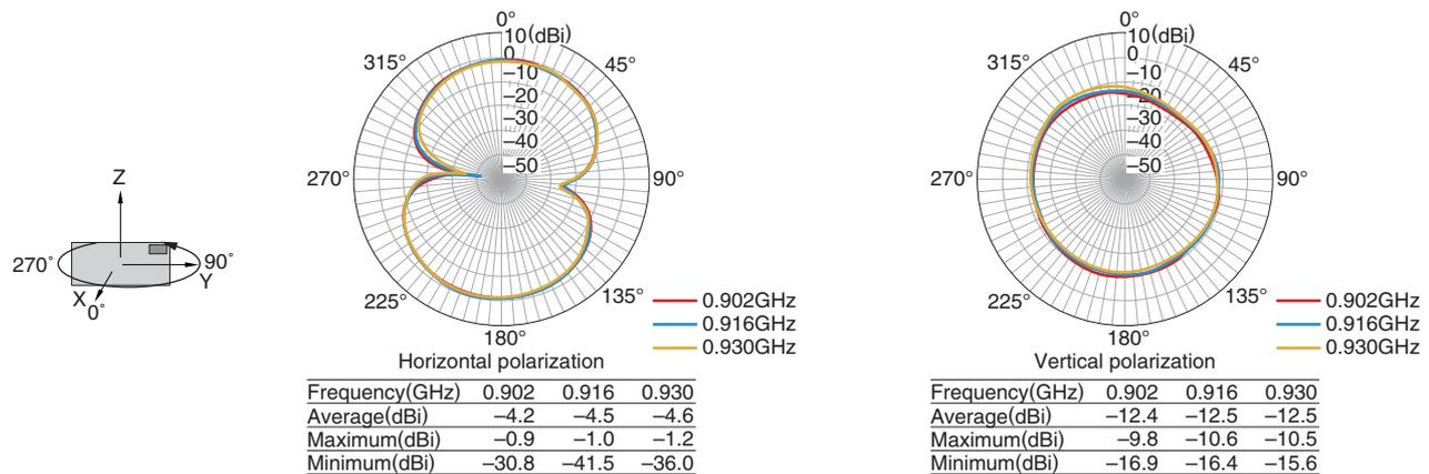
• Tested antenna has been soldered. Evaluation board size is 100x20x1mm.
