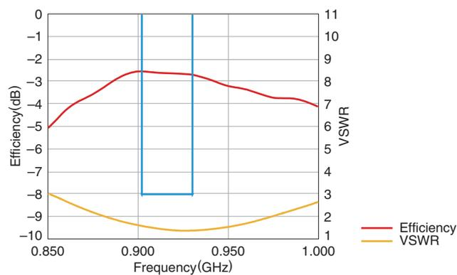
• Tested antenna has been soldered. Evaluation board size is 100x20x1 mm.
