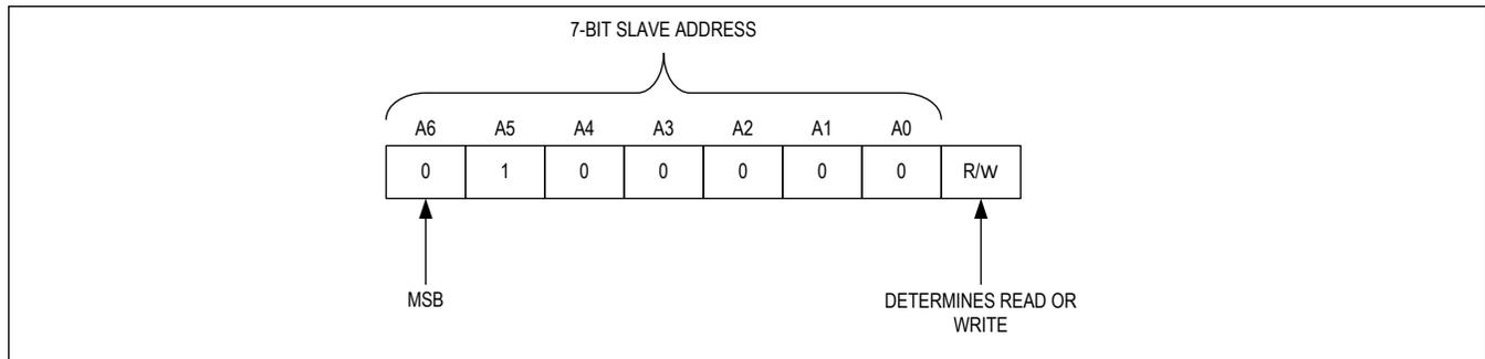
Figure 2. I<sup>2</sup>C Slave Address
