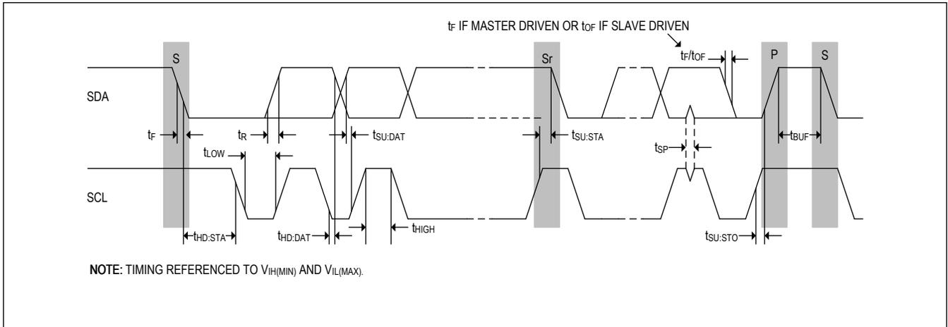
Figure 3. I<sup>2</sup>C Timing Diagram
