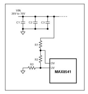
An alternate method used in the application circuits for setting the over-voltage and under-voltage trip points is demonstrated in **Figure 2**. Use  $36.5k\Omega$  for the bottom resistor (R3). R2 and R1 are calculated as follows:
