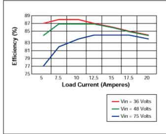
Figure 3. Converter efficiency vs load current.
