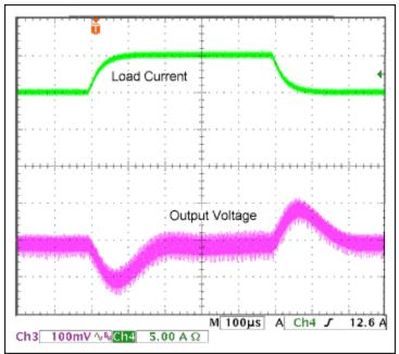
Figure 4. Output voltage deviation for step load increase and decrease. Load current slew rate is approximately 0.1 / $\mu$ S.
