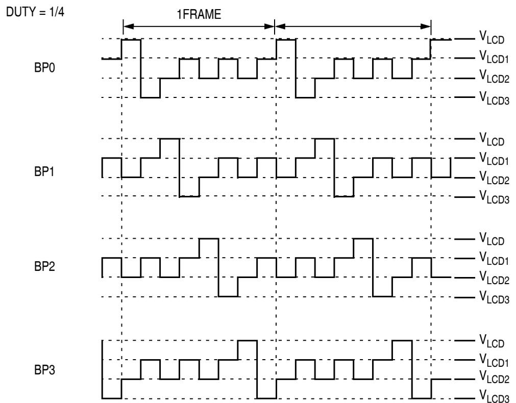
**Figure 16-7. 1/4 Duty LCD Backplane Driver Waveforms**
