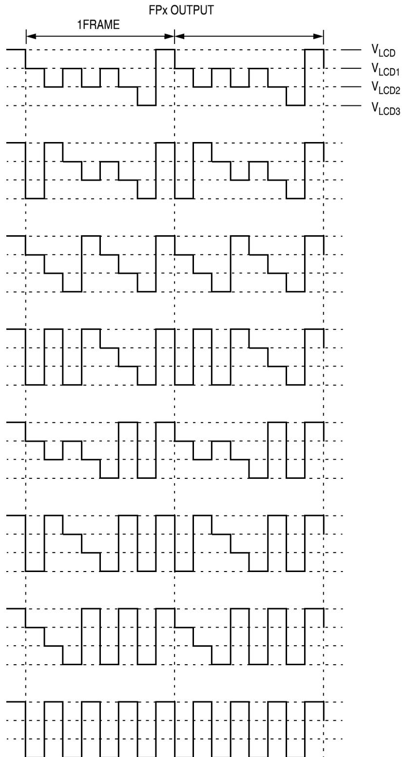
**Figure 16-11. 1/4 Duty LCD Frontplane Driver Waveforms (continued)**
