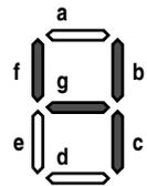
**Figure 16-12. 7-Segment Display Example**
