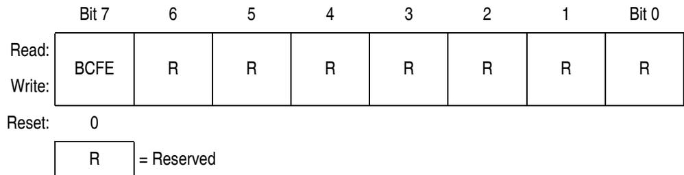
**Figure 9-22. SIM Break Flag Control Register (SBFCR)**
