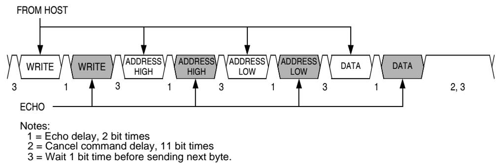
**Figure 10-6. Write Transaction**
