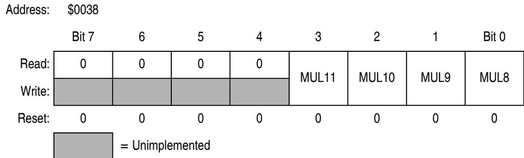
**Figure 8-6. PLL Multiplier Select Register High (PMSH)**
