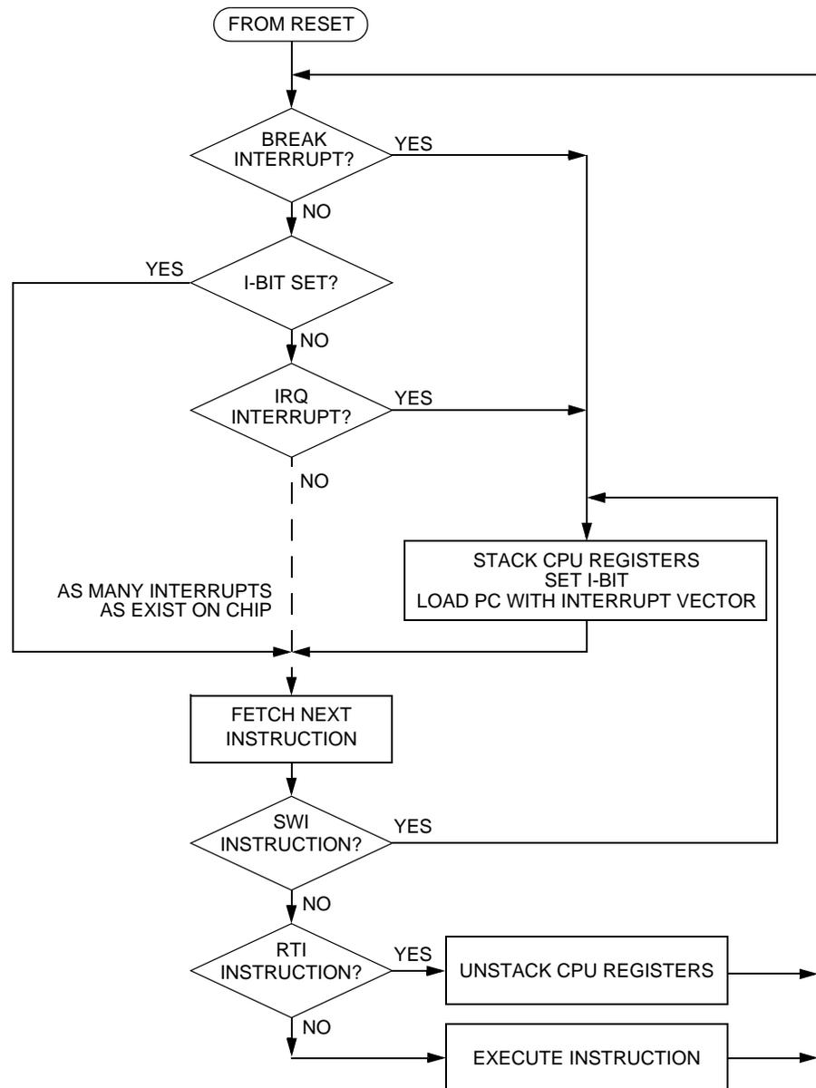
**Figure 9-10. Interrupt Processing**
