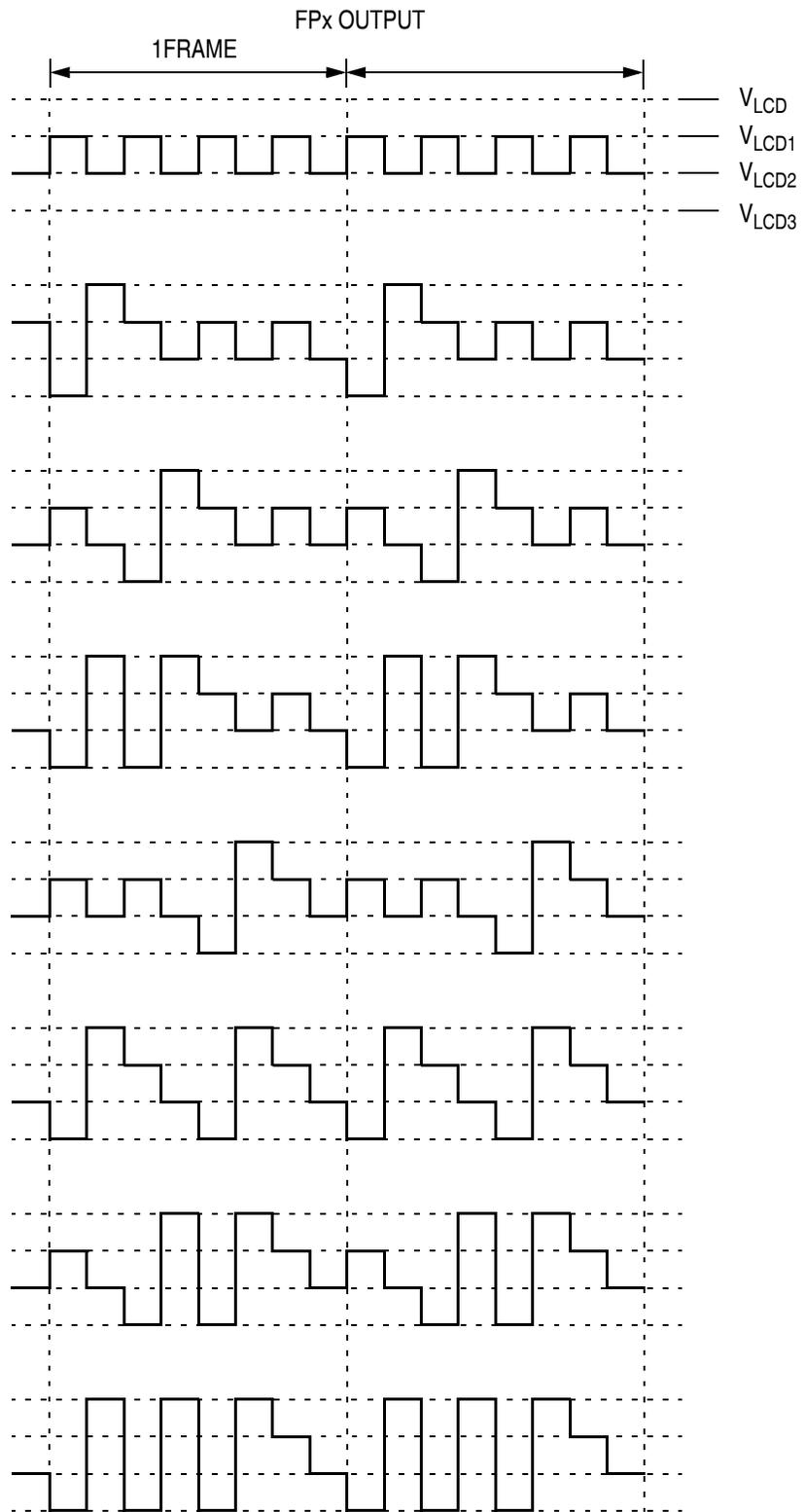
**Figure 16-10. 1/4 Duty LCD Frontplane Driver Waveforms**
