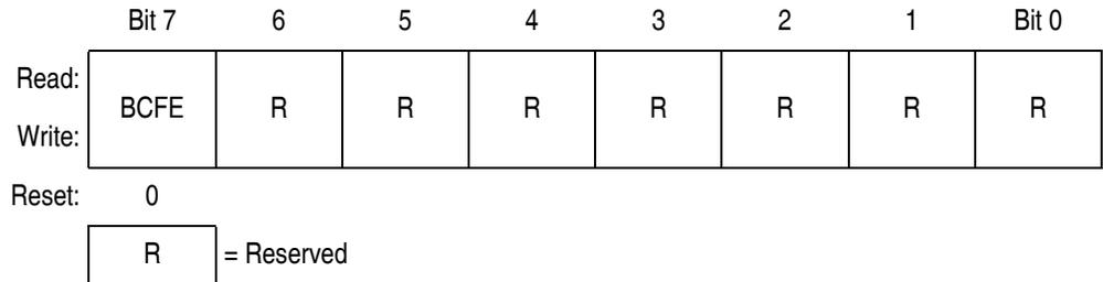
**Figure 22-7. SIM Break Flag Control Register (SBFCR)**
