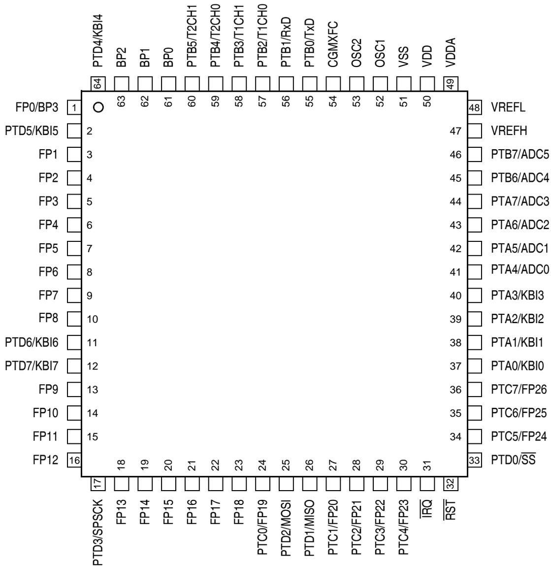
**Figure 1-2. 64-Pin QFP and 64-Pin LQFP Pin Assignment**
