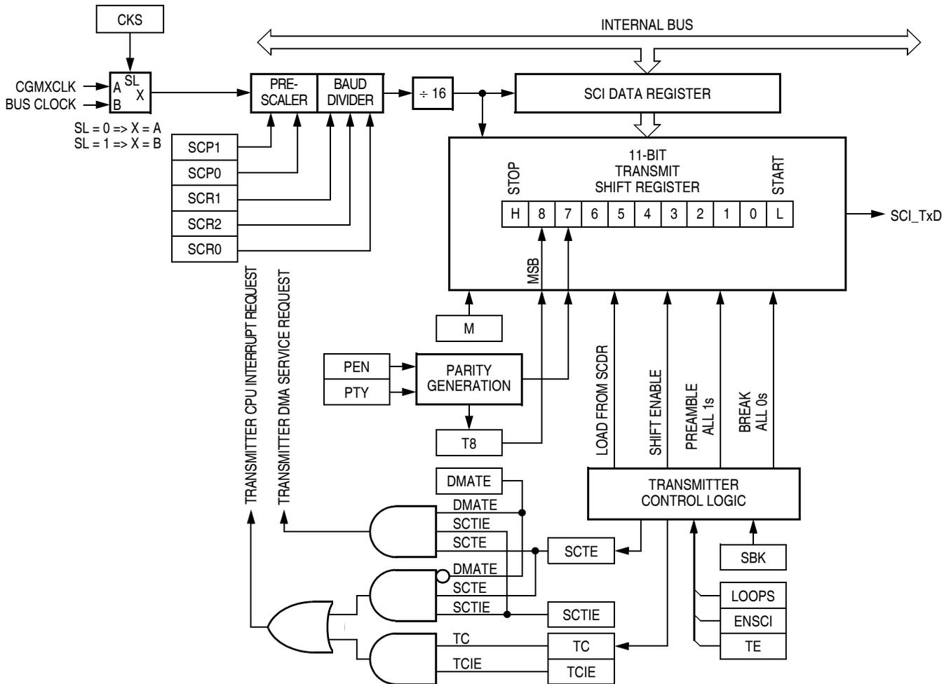
Figure 13-7. SCI Transmitter
