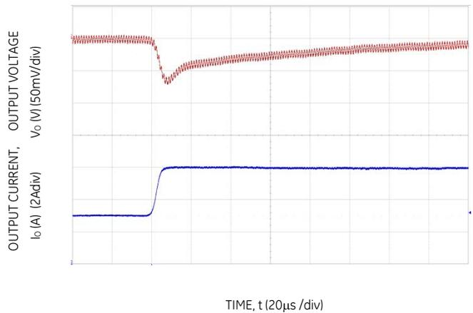
Figure 28. Transient Response to Dynamic Load Change from 50% to 100% at 12V<sub>in</sub>, C<sub>out</sub> = 4x47uF, CTune=2700pF & RTune=300Ω
