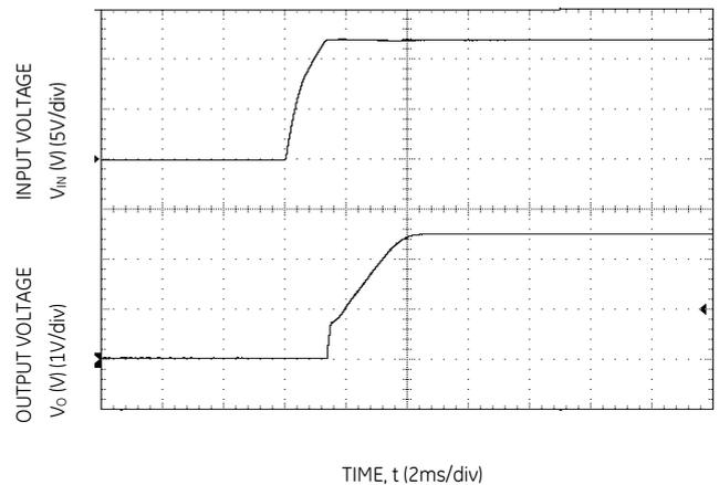
Figure 24. Typical Start-up Using Input Voltage (V<sub>IN</sub> = 12V, I<sub>o</sub> = I<sub>o,max</sub>).
