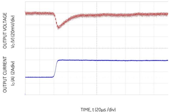
Figure 10. Transient Response to Dynamic Load Change from 50% to 100% at 12Vin,  $C_{out} = 3 \times 47 \mu F + 1 \times 330 \mu F$ ,  $C_{Tune} = 4700 pF$  &  $R_{Tune} = 300 \Omega$
