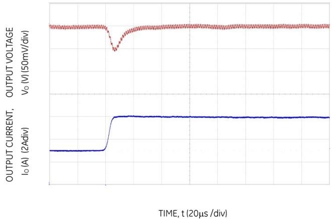
Figure 22. Transient Response to Dynamic Load Change from 50% to 100% at 12V<sub>in</sub>, C<sub>out</sub> = 4x47uF, C<sub>Tune</sub>=2700pF & R<sub>Tune</sub>=300Ω
