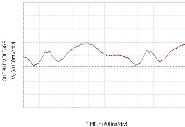
Figure 9. Typical output ripple and noise ( $C_o=1 \times 47 \mu F$  ceramic,  $V_{IN} = 12V$ ,  $I_o = I_{o,max}$ ).
