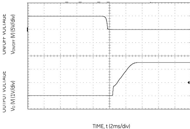
Figure 23. Typical Start-up Using On/Off Voltage (I<sub>o</sub> = I<sub>o,max</sub>).
