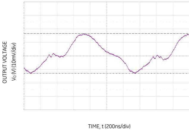
Figure 21. Typical output ripple and noise (C<sub>o</sub>=1x47μF ceramic, V<sub>IN</sub> = 12V, I<sub>o</sub> = I<sub>o,max</sub>).
