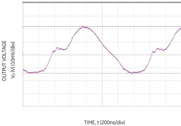
Figure 27. Typical output ripple and noise (C<sub>o</sub>=1x47μF ceramic, V<sub>IN</sub> = 12V, I<sub>o</sub> = I<sub>o,max</sub>).
