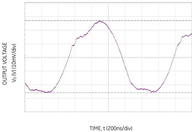
Figure 33. Typical output ripple and noise ( $C_o=1x47\mu F$  ceramic,  $V_{IN} = 12V$ ,  $I_o = I_{o,max}$ ).
