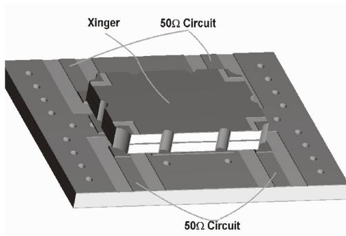
**Figure 3: Component Placement**
