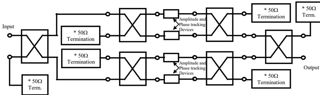
The splitter/combiner networks illustrated above use only 3dB (hybrid) couplers and are limited to binary divisions ( $2^n$  number of splits, where  $n$  is an integer). Splitter/combiner circuits configured this way are known as “corporate” networks. When a non-binary number of divisions is required, a “serial” network must be used. Serial networks can be designed with [3, 4, 5, …,  $n$ ] splits, but have a practical limitation of about 8 splits.
