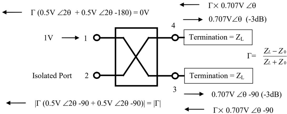
The reflection property of common mismatches in 3dB couplers is very beneficial to the operation of many networks. For instance, when splitter/combiner networks are employed to increase output power by paralleling transistors with similar reflection coefficients, input return loss is not degraded by the mismatch of the transistor circuit. The reflections from the transistor circuits are directed away from the input to the termination at the isolated port of the coupler.
