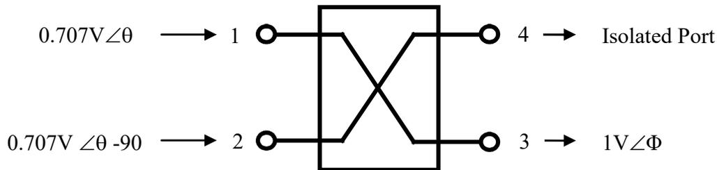
3dB couplers have applications in circuits which require splitting an applied signal into 2, 4, 8 and higher binary outputs. The couplers can also be used to combine multiple signals (inputs) at one output port. Some splitting and combining schemes are illustrated below:
