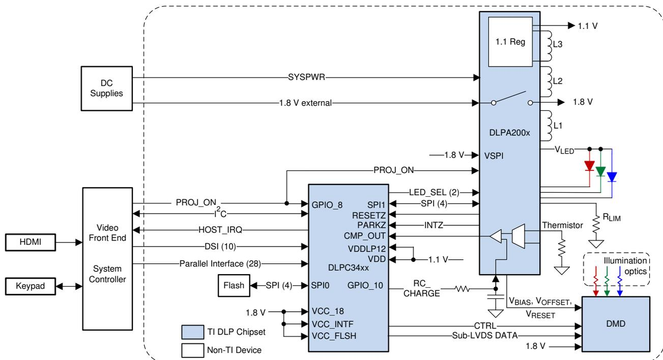
Figure 8-1. Typical Simplified Application Schematic (using DLPA200x)
