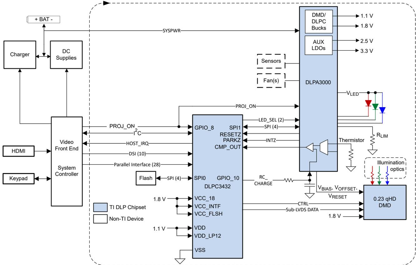
**Figure 8-2. Typical Simplified Application Schematic (using DLPA3000)**
