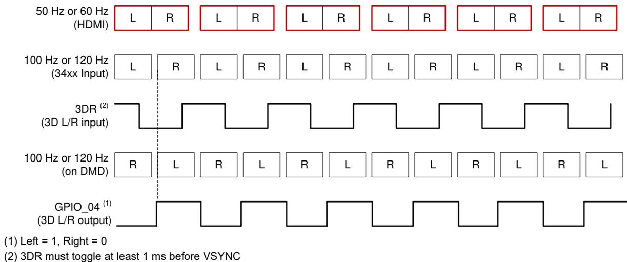
**Figure 7-1. 3D Display Left and Right Frame Timing**
