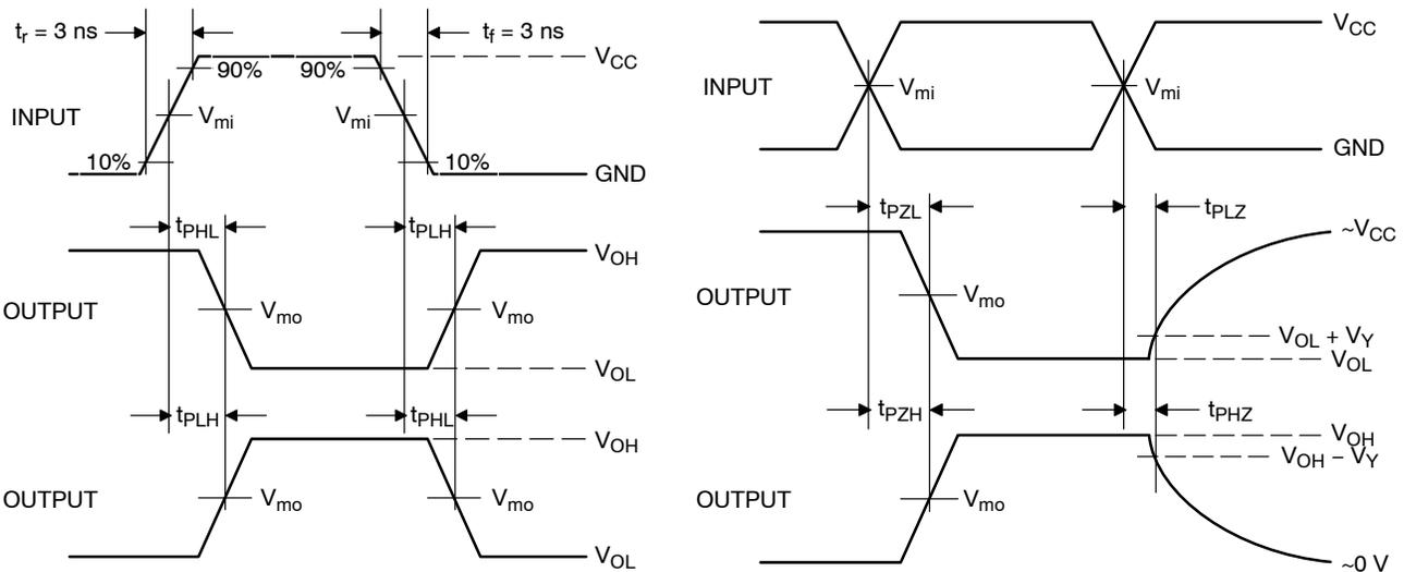
**Figure 4. Switching Waveforms**
