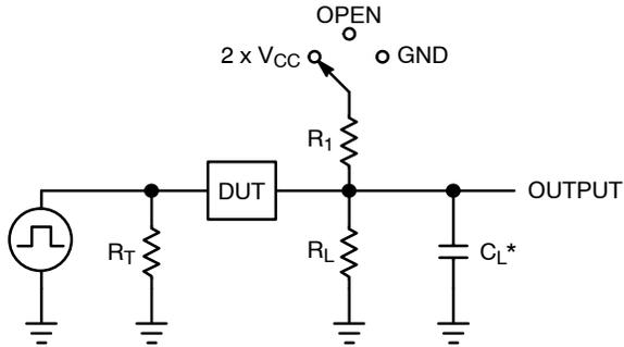
C<sub>L</sub> includes probe and jig capacitance
