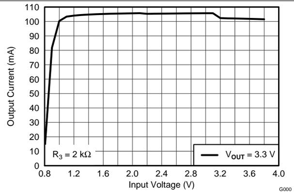
Figure 2. Maximum Output Current vs Input Voltage
