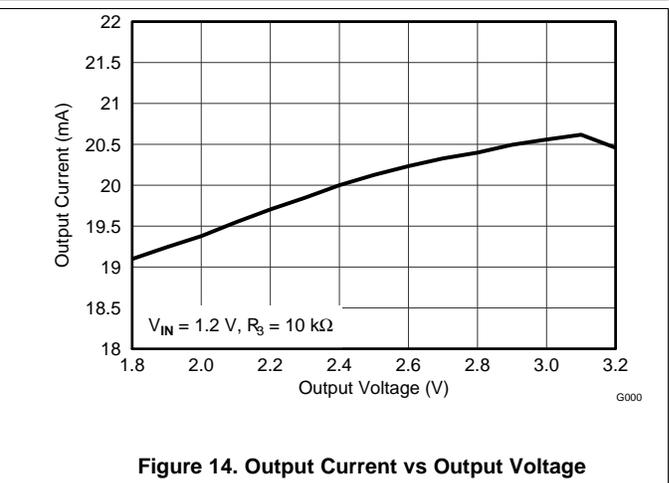
Figure 14. Output Current vs Output Voltage
