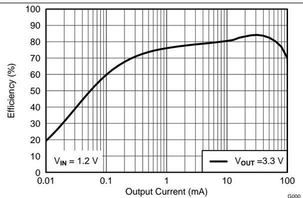
Figure 4. Efficiency vs Output Current
