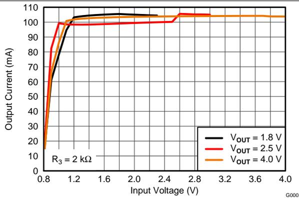
Figure 1. Maximum Output Current vs Input Voltage
