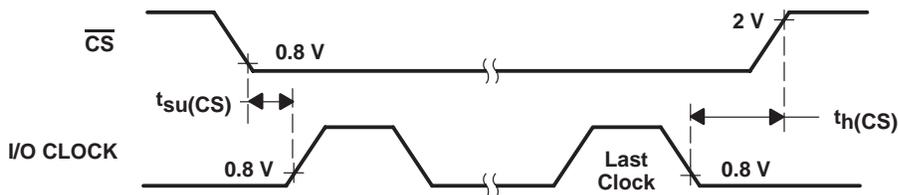
Figure 6.  $\overline{\text{CS}}$  and I/O CLOCK Voltage Waveforms†
