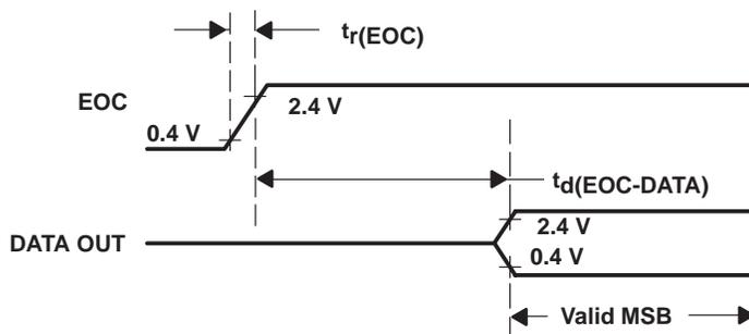
Figure 9. EOC and DATA OUT Voltage Waveforms
