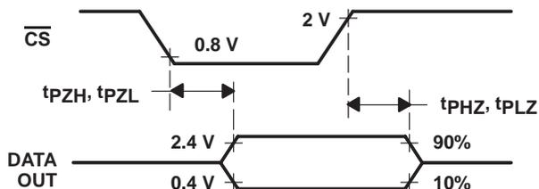
**Figure 4. DATA OUT to Hi-Z Voltage Waveforms**
