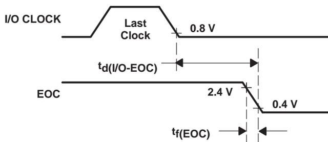
Figure 8. I/O CLOCK and EOC Voltage Waveforms
