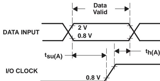
**Figure 5. DATA INPUT and I/O CLOCK Voltage Waveforms**
