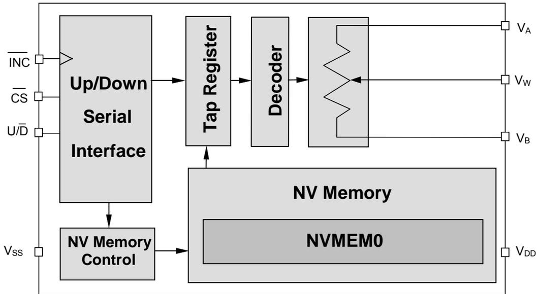
FIGURE 1 – WMS7140 BLOCK DIAGRAM (Rheostat Mode)
