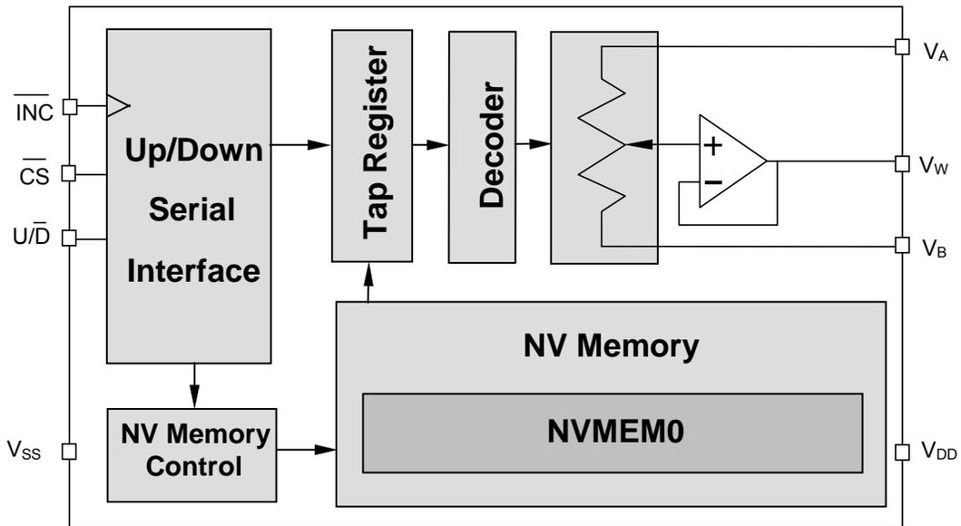
FIGURE 2 – WMS7141 BLOCK DIAGRAM (Divider Mode)
