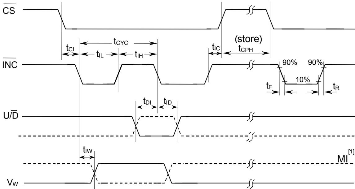
**FIGURE 3 –WMS7140/1 TIMING DIAGRAM**
