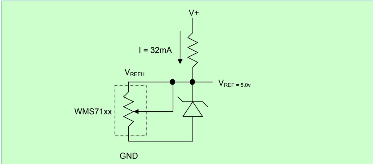
FIGURE 7 – WMS7140/1 TRIMMING VOLTAGE REFERENCE
