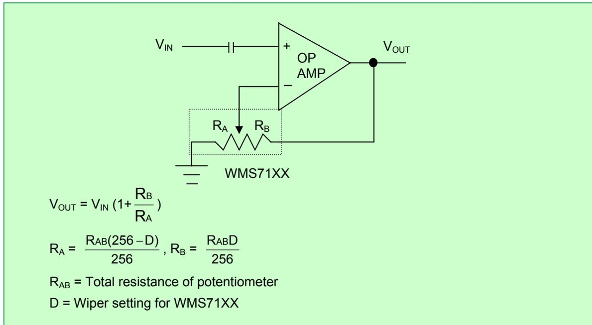
FIGURE 6 – PROGRAMMABLE NON-INVERTING GAIN AMPLIFIER USING THE WMS7140/1
