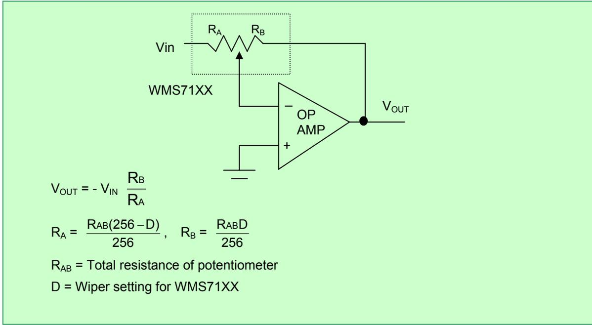
FIGURE 5 – PROGRAMMABLE INVERTING GAIN AMPLIFIER USING THE WMS7140/1
