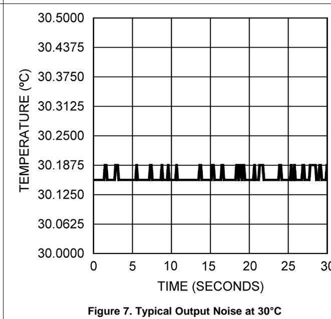
Figure 7. Typical Output Noise at 30°C
