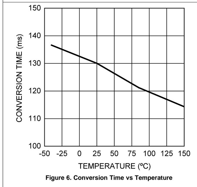
Figure 6. Conversion Time vs Temperature
