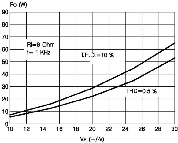
Figure 5. Distortion vs. output power
