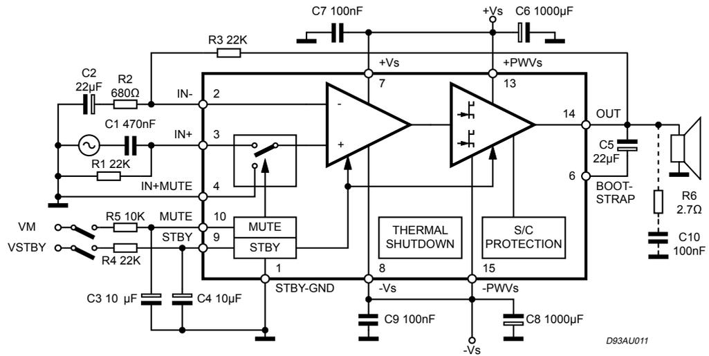
Note: The Boucherot cell R6, C10, normally not necessary for a stable operation it could be needed in presence of particular load impedances at  $V_s < \pm 25V$ .
