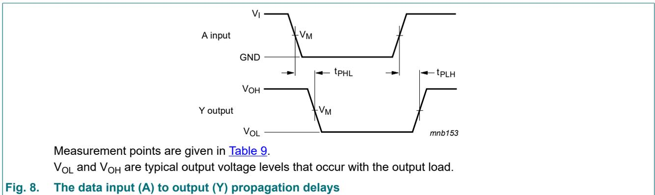
**Fig. 8. The data input (A) to output (Y) propagation delays**
