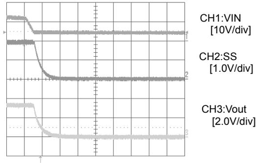
•EN start up waveform Rload = 3.3 $\Omega$  [1msec/div]
