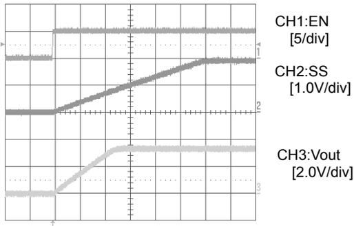
•EN stop waveform Rload = 3.3 $\Omega$  [0.2msec/div]
